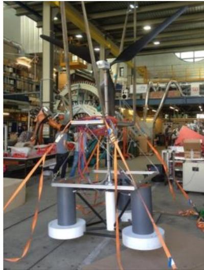
Figure 7 – Pendulum tests for mass identification.
