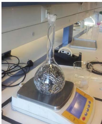
Figure 28 – Measurement of the water displaced volume for one chain
