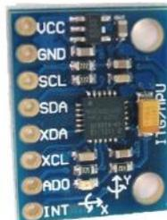
Figure 56 – MPU-6050 six-axis gyroscope + accelerometer.
