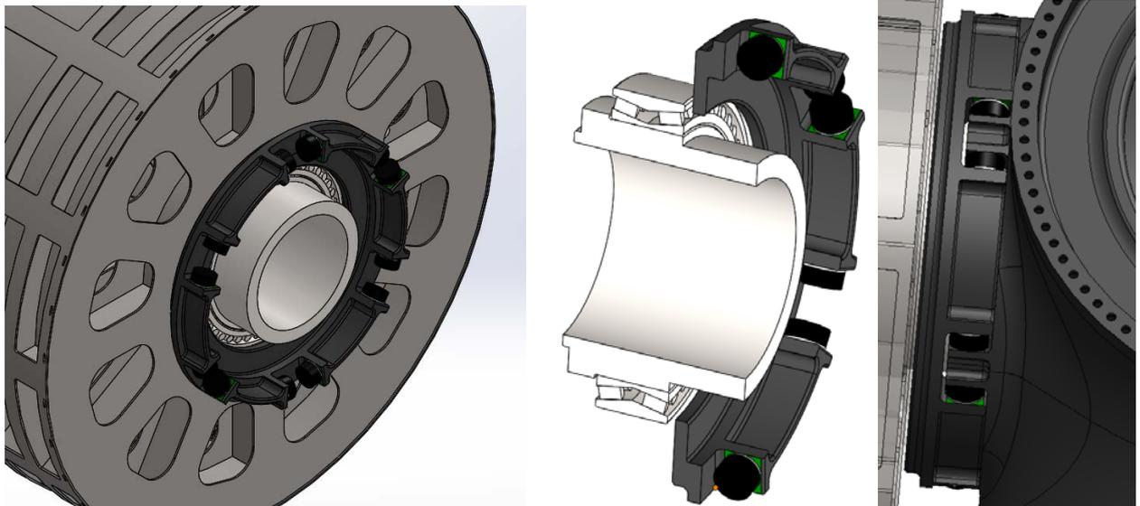
The hydraulic pads transmit the torque by the stiff behaviour in the pad normal direction but the pads are compliant in the other directions isolating the generator from the relative deflections between the rotor hub and kingpin.
