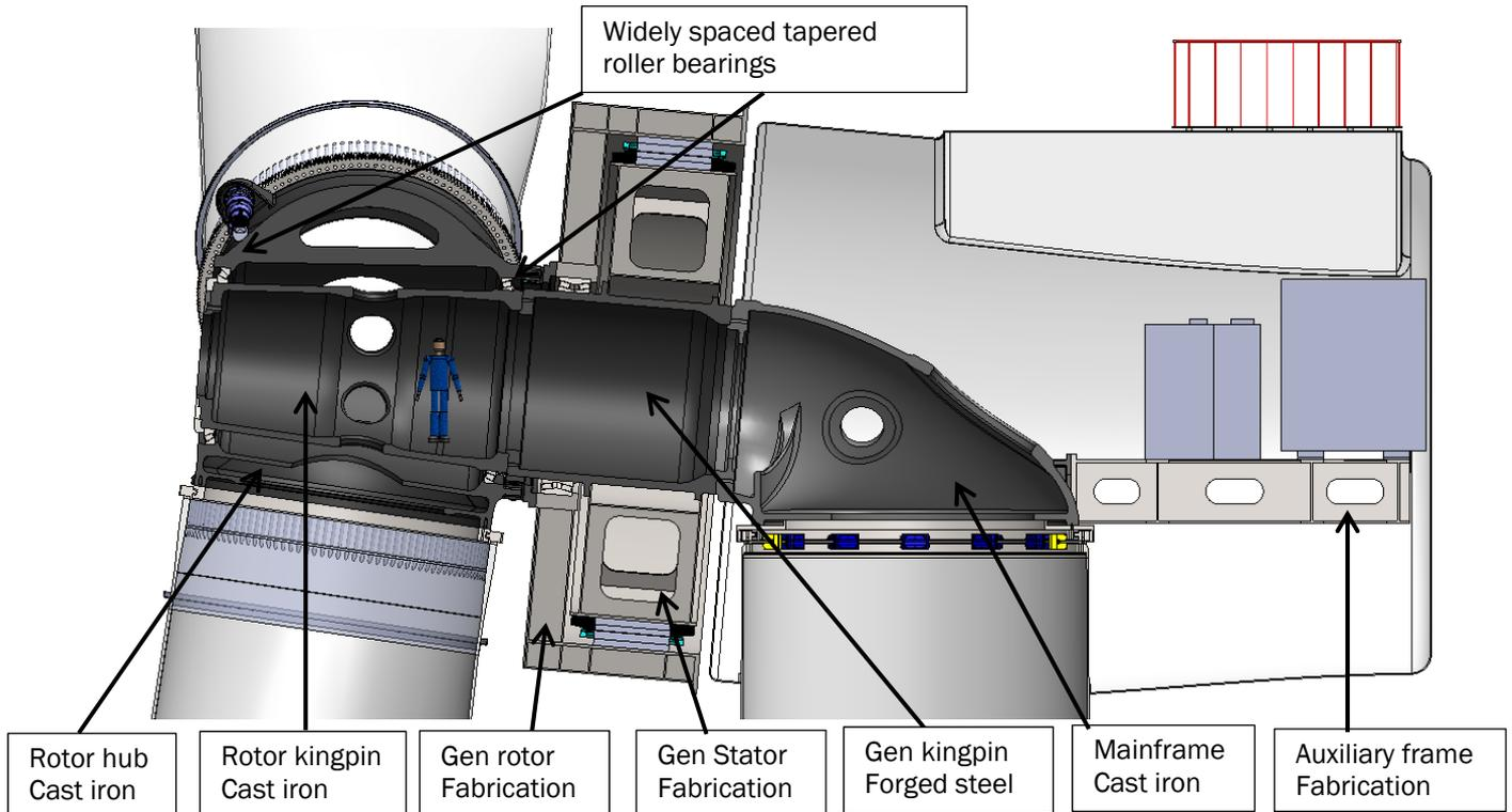
Also in this concept like in SCDD1, the shape of the rotor king pin and generator kingpin are chosen as large as possible utilising strength of the component and efficient bolted connections.
