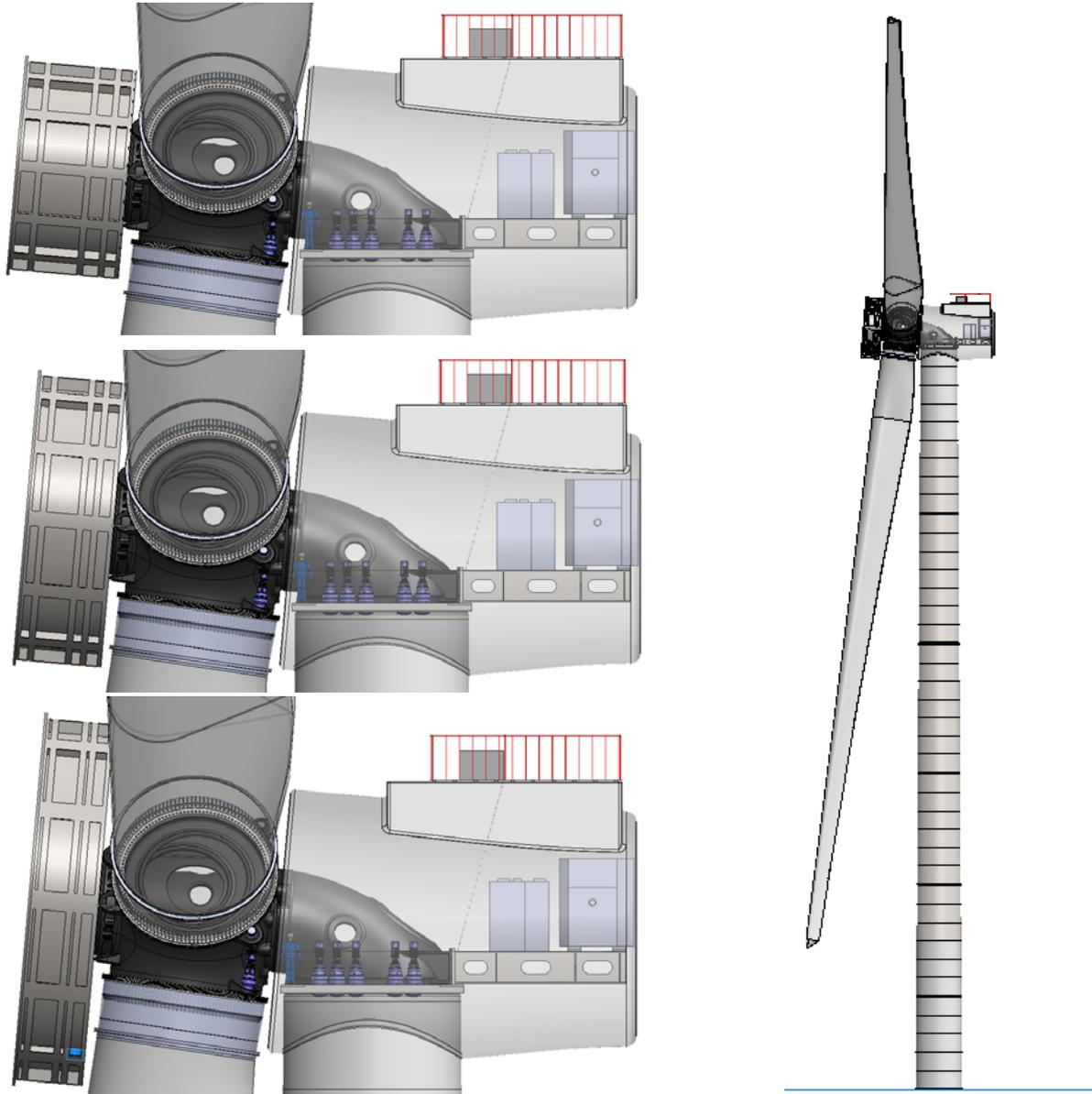
For all three generator configurations there is clearance between the generator structure and blade although for SCDD3 the clearance is small.
