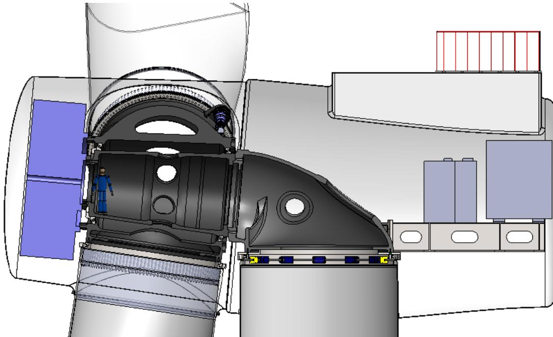
The PDD generator is more compact than the SCDD generator design and is easy to integrate within the rotor spinner cover.
