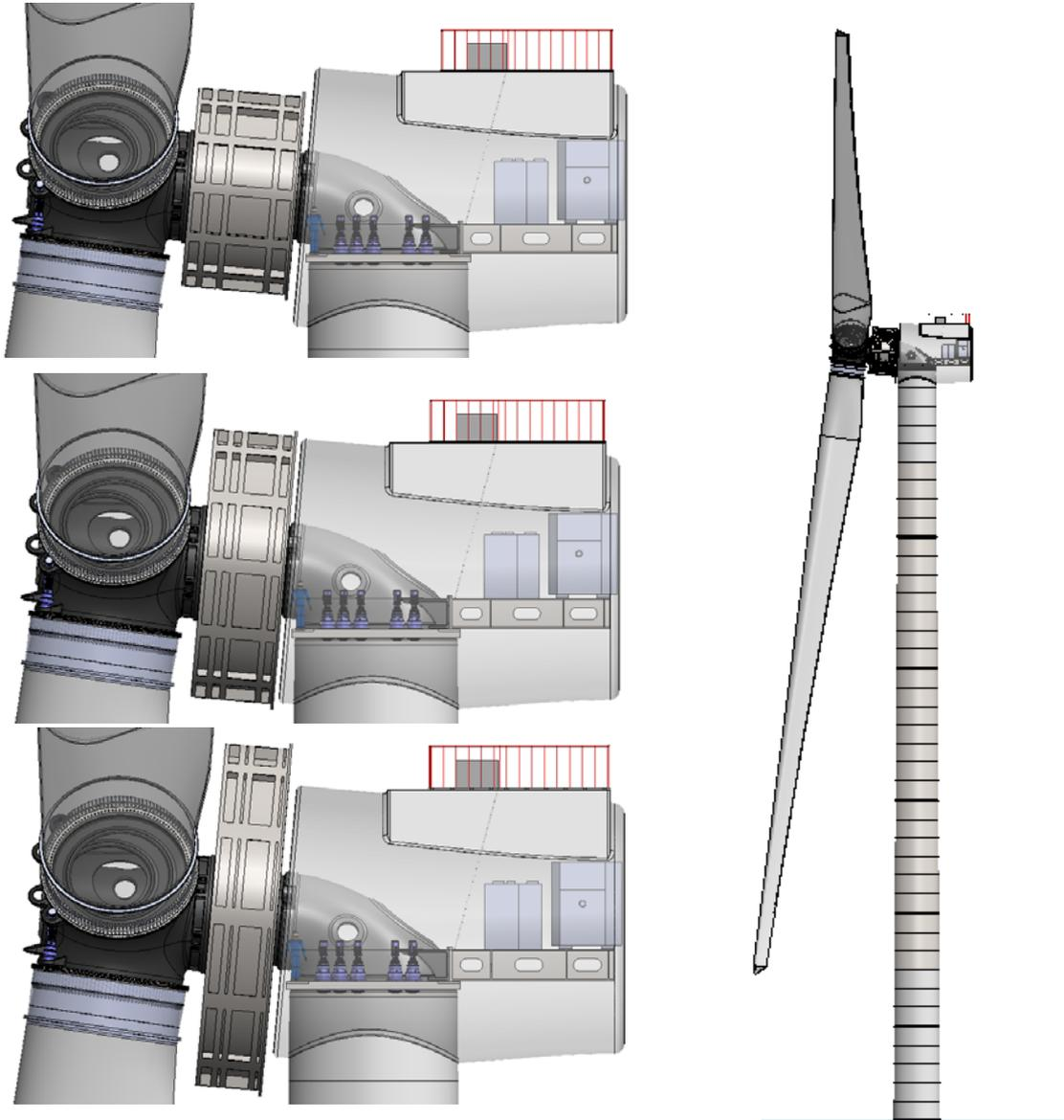
For all three configurations there is sufficient clearance between the generator and blades due to the blade cone angle and there is also enough space between the generator and the tower because of the drivetrain tilt angle.
