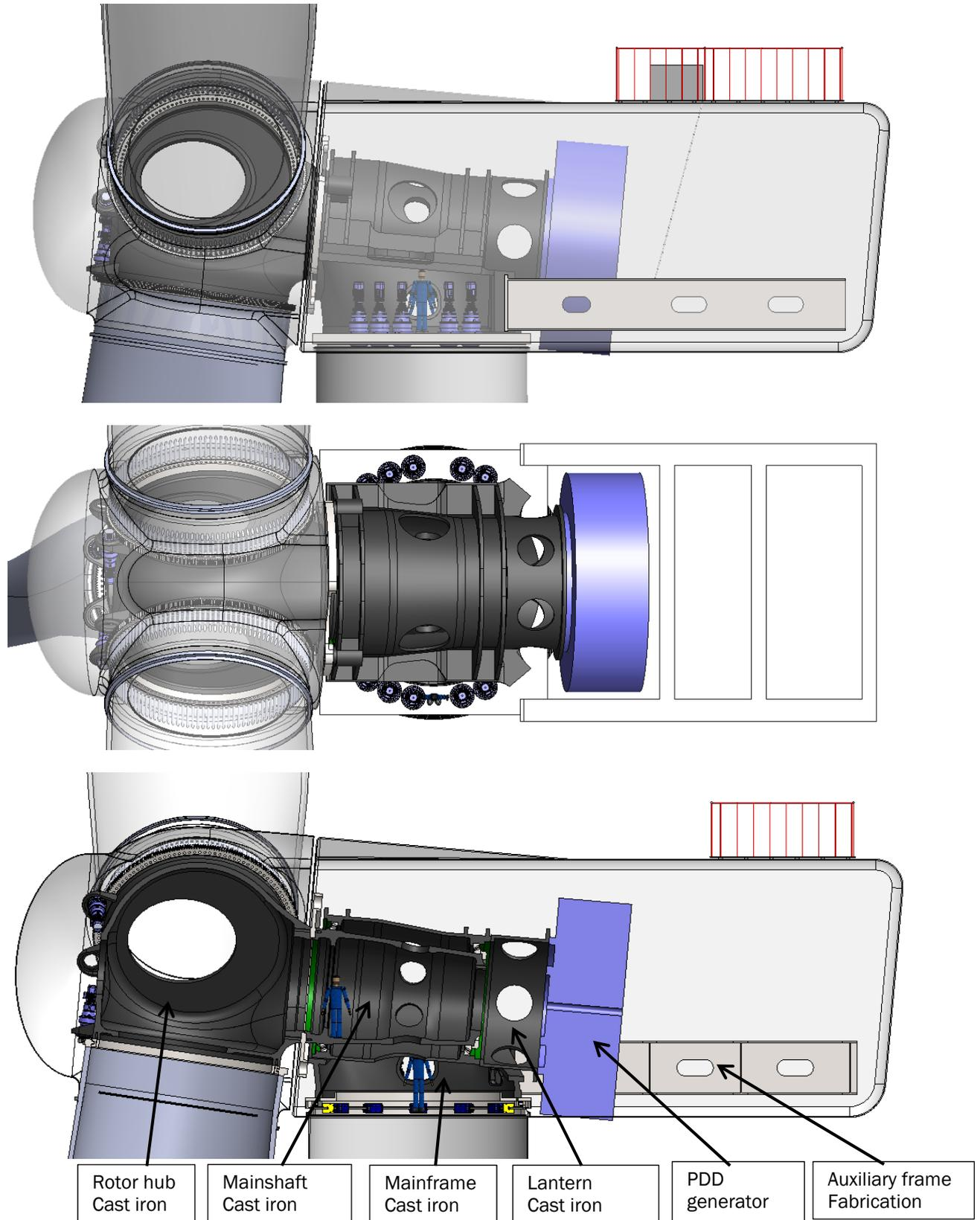
The size of the generator is still very large in comparison with a conventional gearbox or generator and can therefore not be easily located anywhere above the tower. In this relative conventional concept layout the generator must be located further backward and fall behind the tower top.
