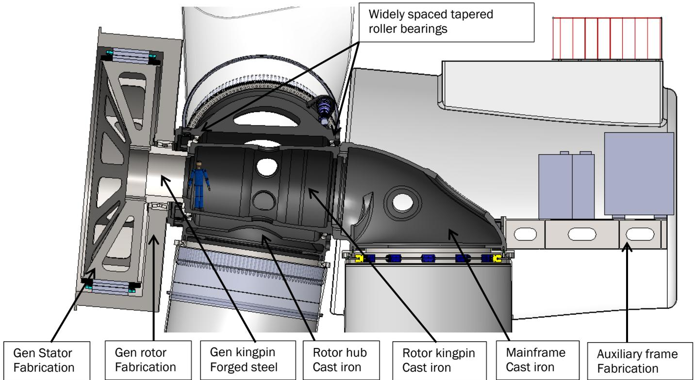
The shape of the rotor king pin is deliberately chosen as large as possible maximising components strength and resulting in an efficient loaded bolted connection to the mainframe. The upwind diameter of the rotor kingpin should be sufficient to design a strong enough bolted connection to the generator.
