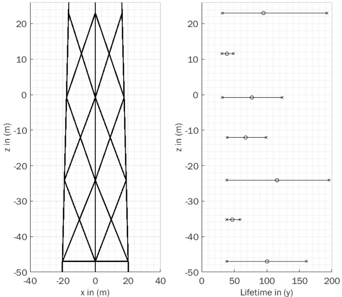
Fig. 10: Hybrid joint lifetimes of ideal jacket for each joint layer. Crosses show the minimum and maximum lifetimes on each layer, circles the corresponding mean lifetime.
