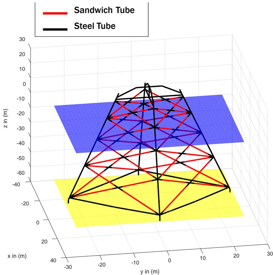
**Fig. 1: INN WIND.EU 10 MW reference jacket with steel legs and sandwich braces**
