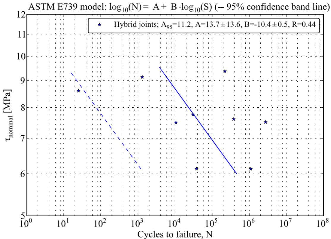
Fig. 6: Experimental S-N curve for hybrid joints
