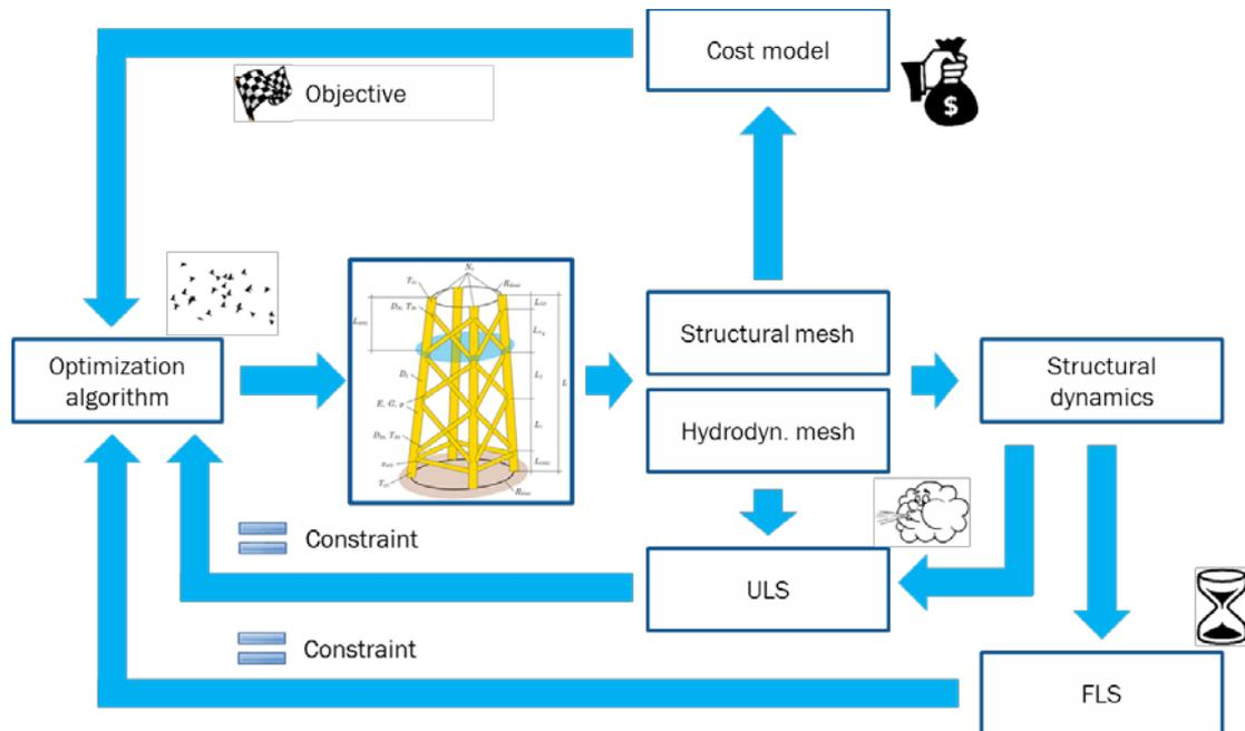
Fig. 7: Scheme of the approach for jacket optimization
