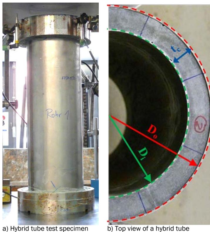
Fig. 4: Hybrid tube test specimen a) and cross section b)
