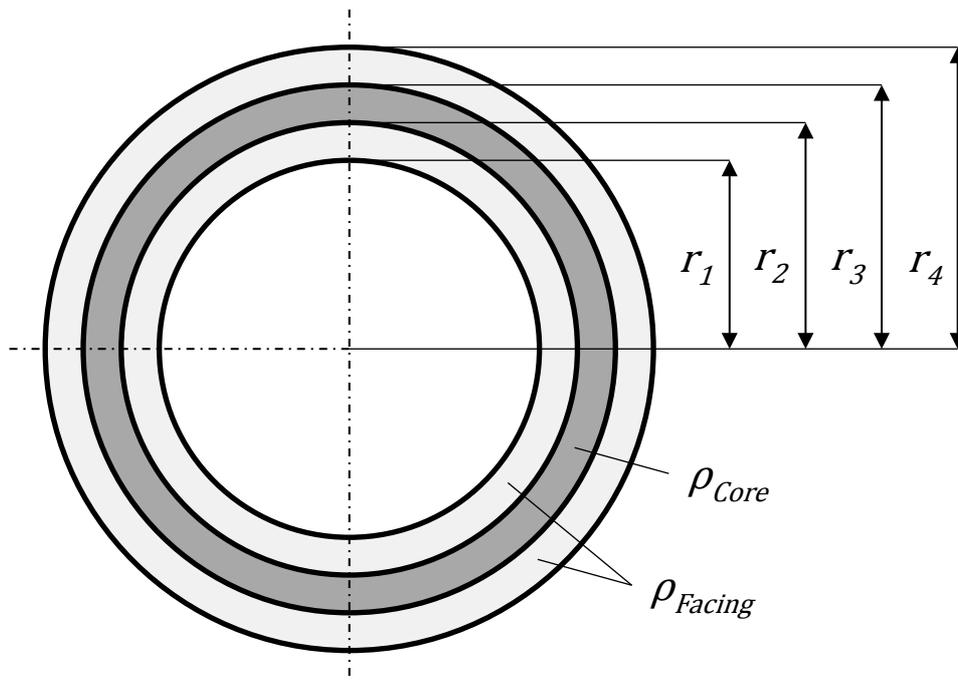
Fig. 3: Cross-section of sandwich tube with corresponding quantities
