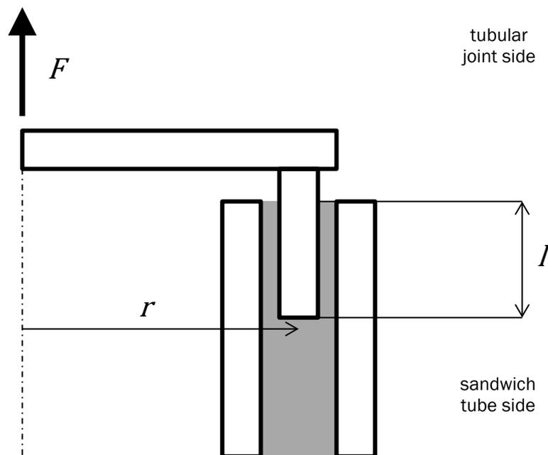
Fig. 5: Schematic illustration of the hybrid joint concept with measures used for shear stress calculation
