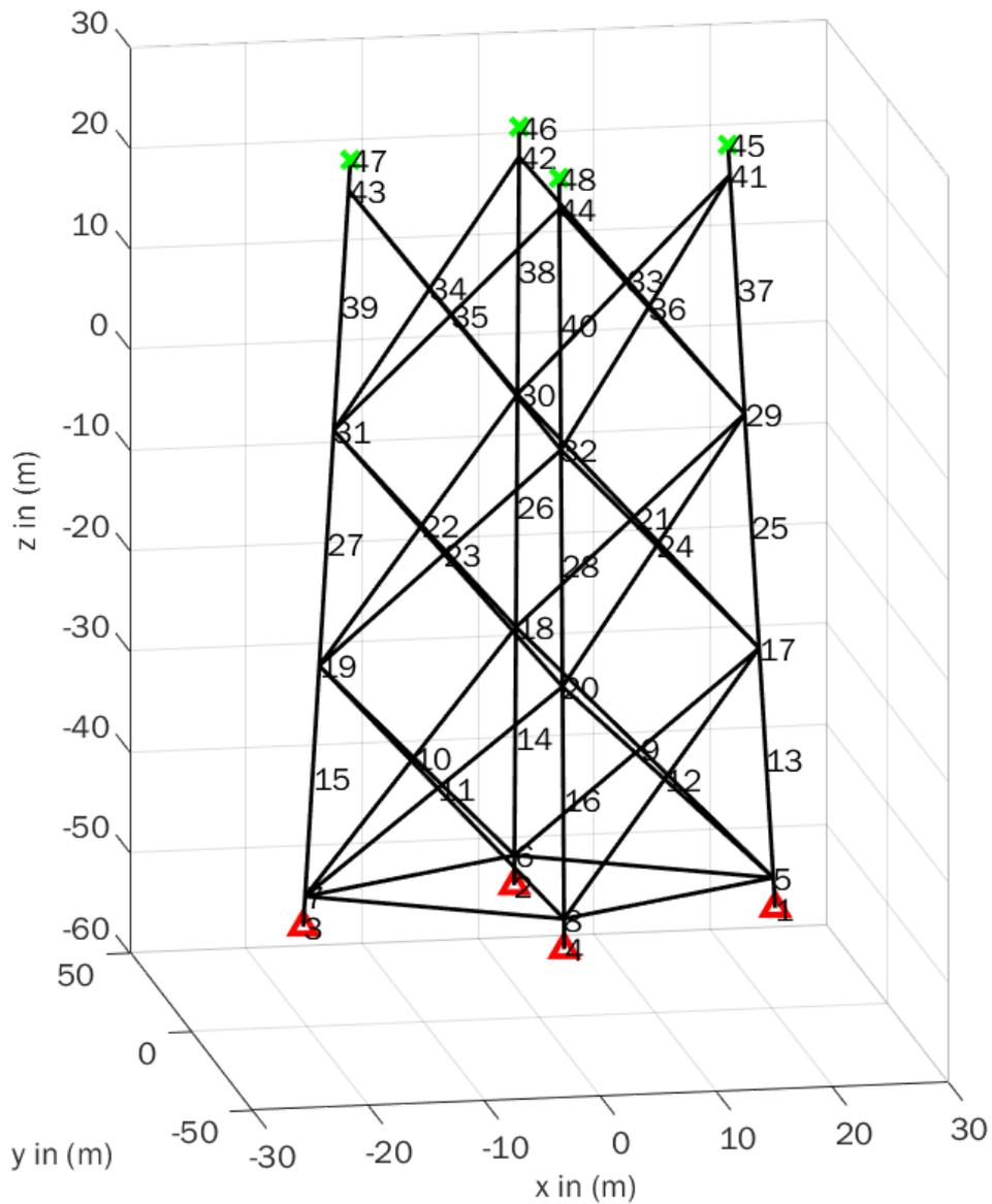
Fig. 9: Topology of ideal jacket with joint numbers (red triangles depict base joints, green crosses depict interface joints)
