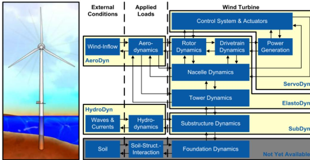
Fig. 2: Modular structure of aero-hydro-servo-elastic simulation framework FAST [18]
