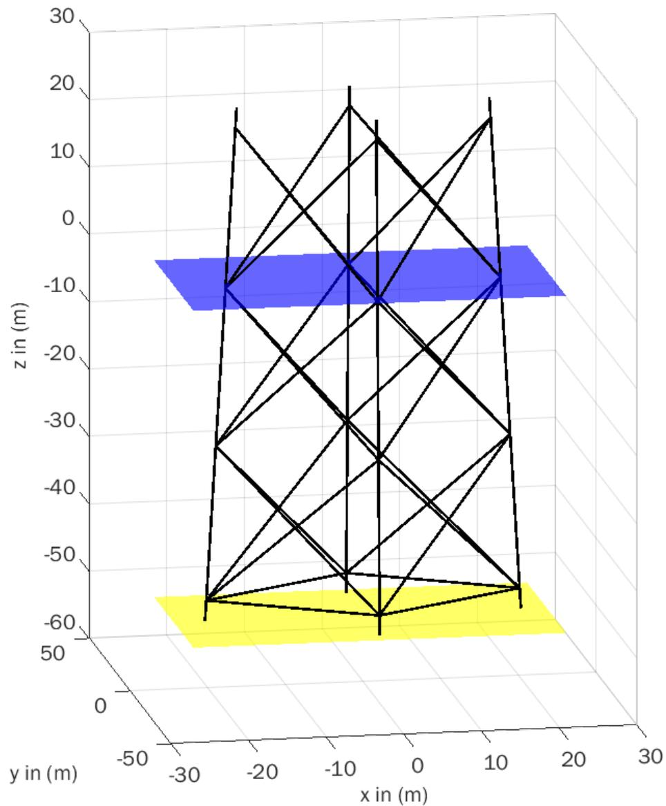
Fig. 8: Topology of ideal hybrid-type jacket design obtained by optimization approach (blue: mean sea level layer, yellow: soil layer)
