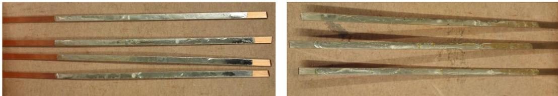
Figure 3.11: Pre-soldering of copper (left) and nickel (right) sides of the  $MgB_2$  superconductor.
