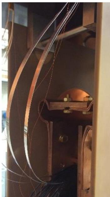
Figure 4.6: HTS tapes between the coil and the second temperature stage.
