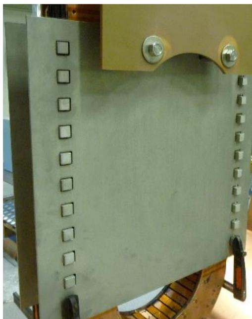
Figure 4.1: Mechanical support mounted on the coil.
