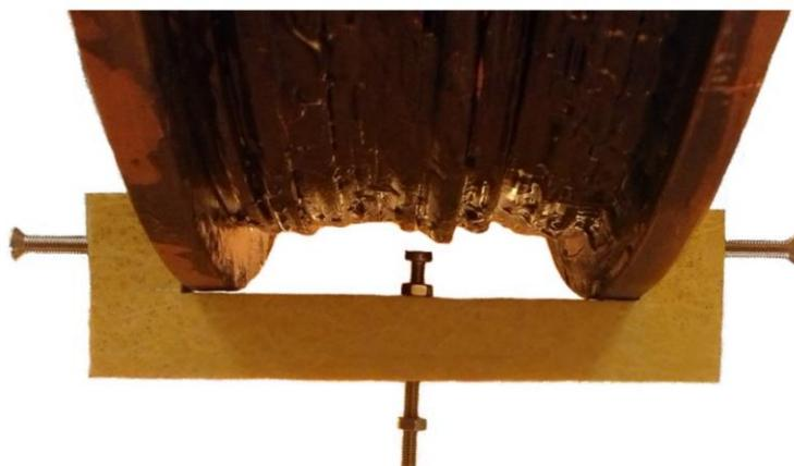
Figure 5.3: Sample holder for bottom Cernox sensor at the bottom of the cryostat furthest away from the cold head.
