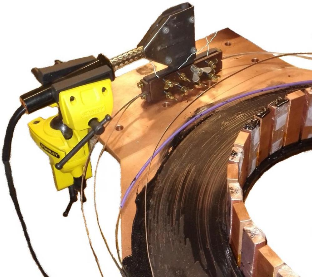
Figure 3.10: The first and second coil soldered together.
