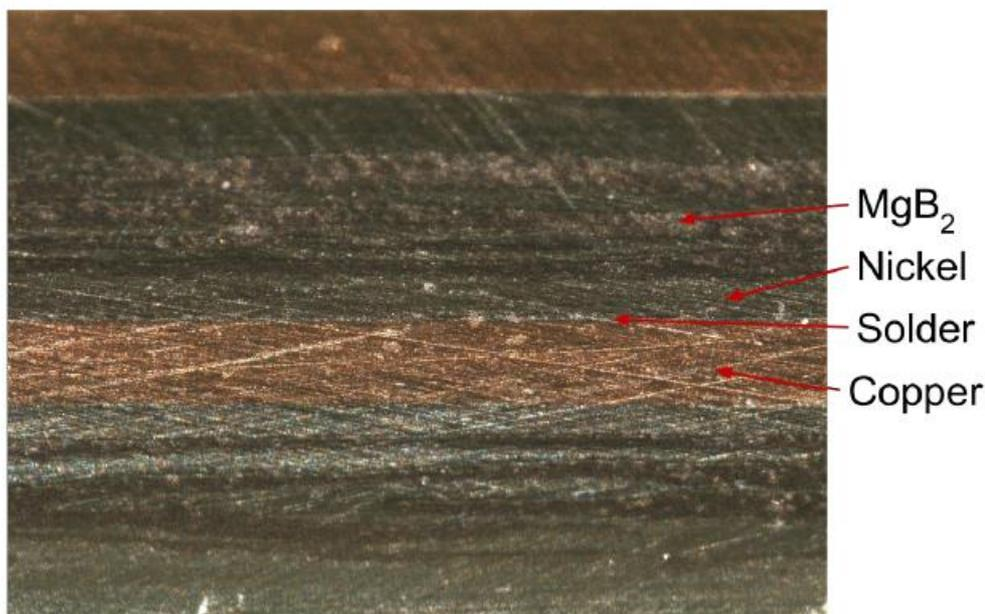
Figure 3.13: Optical microscope cross-section view of soldered joint.
