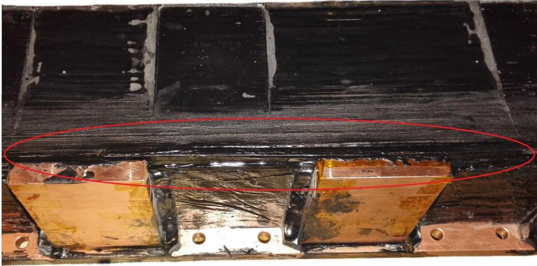
Figure 3.9: The pieces of superconductor that were placed between the tenth coil and the copper teeth.
