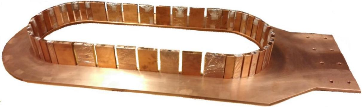
Figure 3.6: The bottom of the thermal interface with all the copper teeth mounted on the inner edge.
