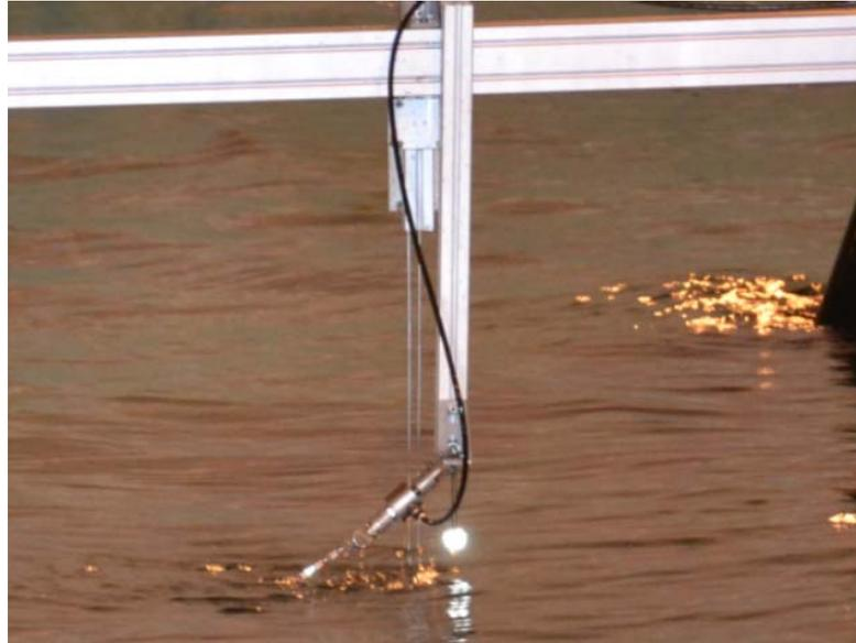
**Figure 4.3: Load cell for the measurement of the tension**
