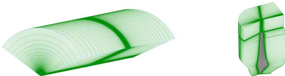
Figure 67 – Background (left) and blade (right) grid of the one third model in FLOWer
