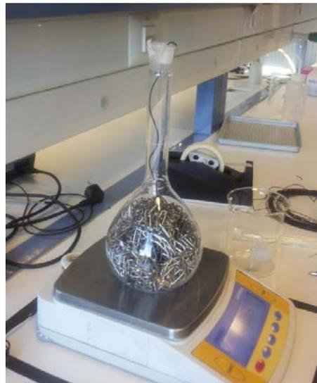
Figure 4.5: Measurement of the displaced volume of the chain
