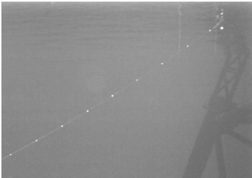
**Figure 4.4: Chain with markers to measure the motions**
