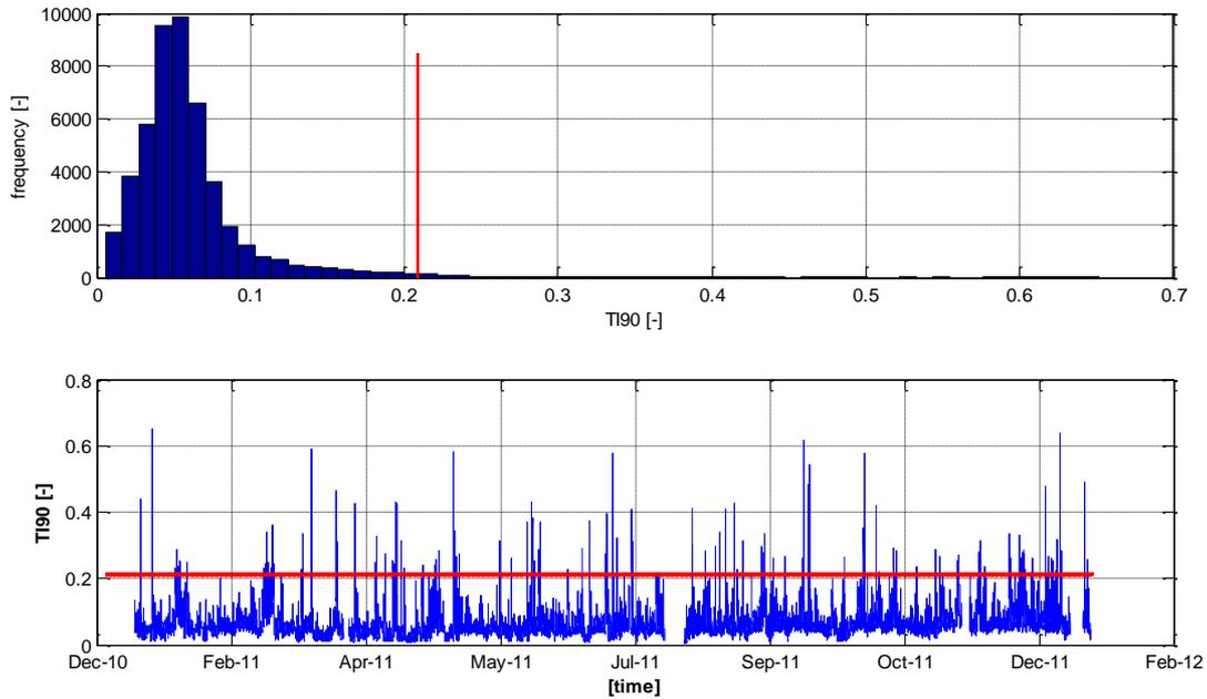
**Figure 31:** Frequency distribution and time series of the turbulence intensity TI at FINO 3 during year 2011, value of four times  $\sigma$  of TI marked with red line.
