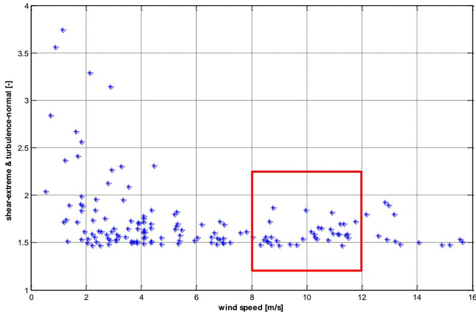
**Figure 35:** Extreme wind shear (selected for normal TI) in dependence to the wind speed at FINO 3, exemplary wind condition 2 marked with red box.
