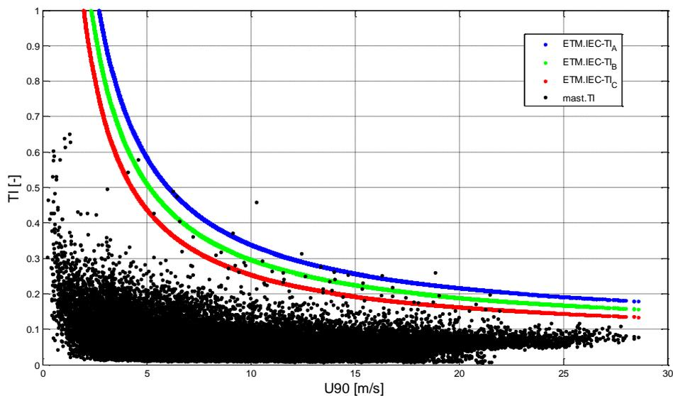
**Figure 22:** Turbulence intensity TI of the wind speed at FINO 3 in 90 m height and the theoretical values of the Extreme Turbulence Model (IEC 61400-1 Ed.3).
