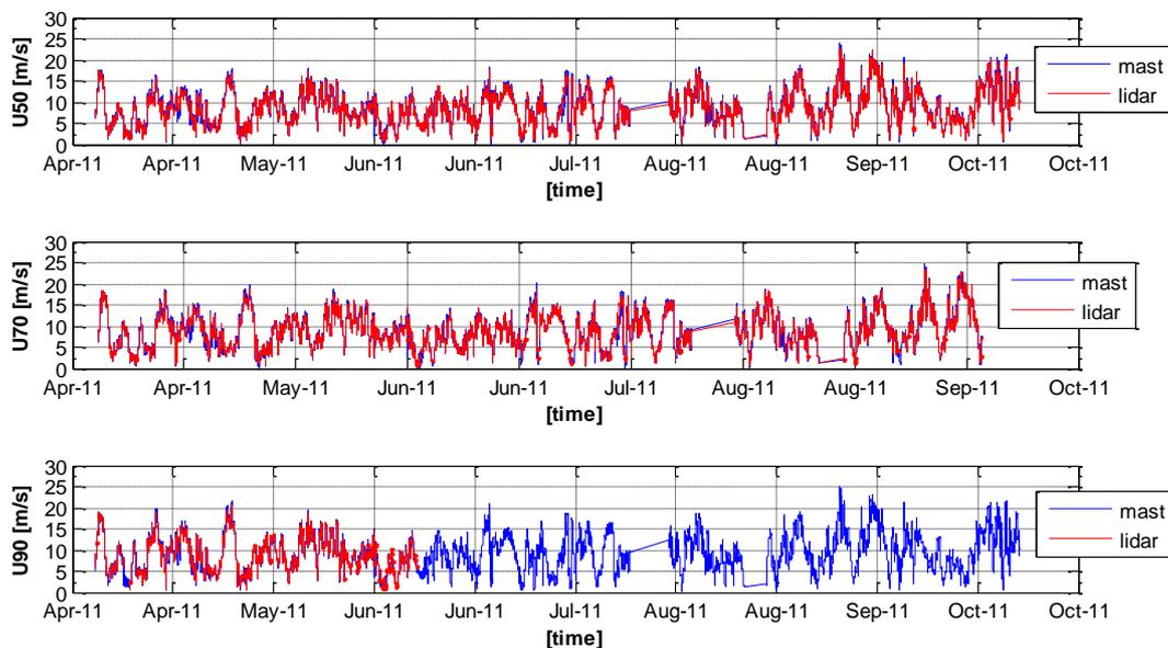
Figure 25: Comparison of the time series of the LiDAR data with mast data in 50 m (top), 70 m (middle) and 90 m (bottom) height at FINO 3.
