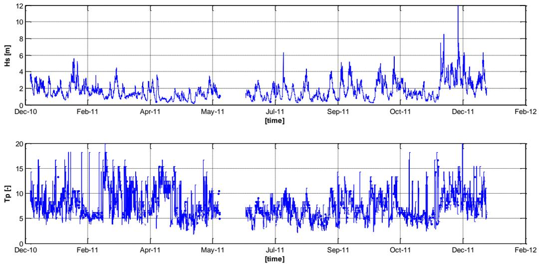
**Figure 27:** Time series of the significant wave height  $H_s$  (top) and the peak wave period  $T_p$  (bottom) measured by the buoy at FINO 3 during year 2011.
