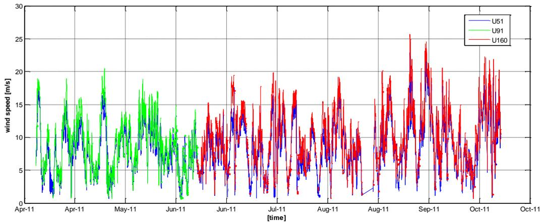
Figure 24: Time series of the LiDAR data in 51 m, 71 m and 91 m height at FINO 3.
