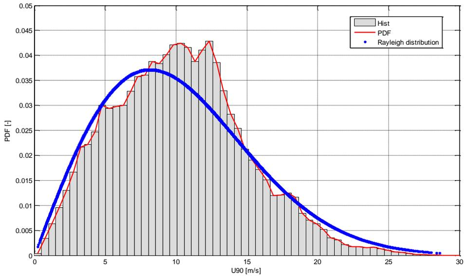
**Figure 12:** Frequency distribution, PDF and Rayleigh distribution of the wind speed at FINO 3 in 90 m height for year 2011.
