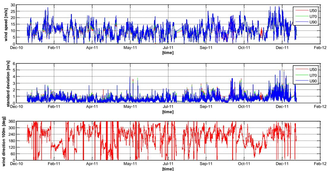
**Figure 11:** Time series of the wind speed (top), standard deviation of the wind speed (middle) in 50 m, 70 m and 90 m height and wind direction (bottom) in 100 m height at FINO 3 during year 2011.
