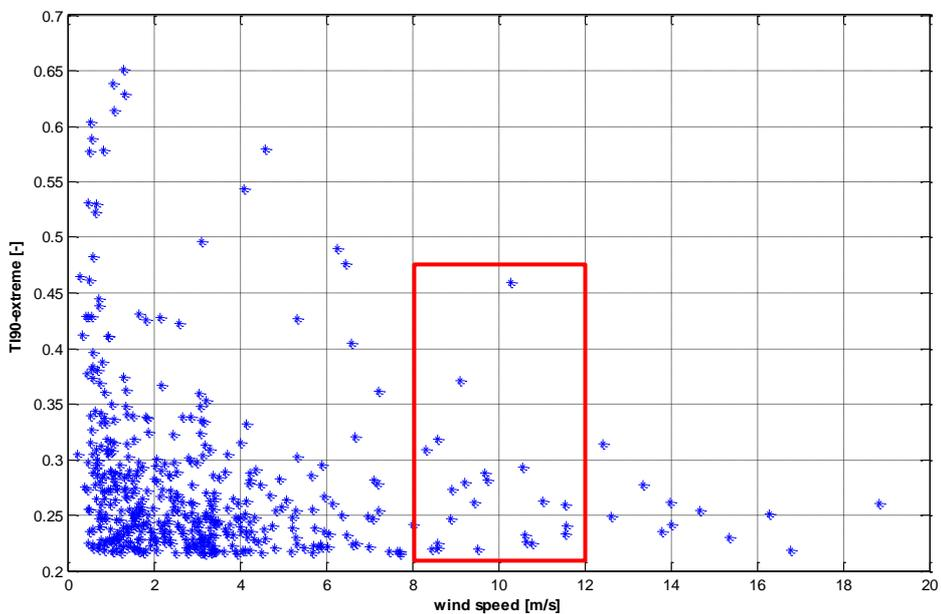
**Figure 32:** Extreme turbulence intensities in dependence to the wind speed at FINO 3, exemplary wind condition 1 marked with red box.
