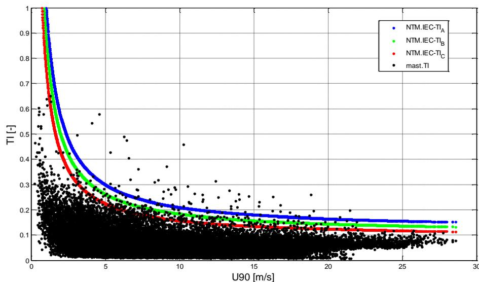
**Figure 20:** Turbulence intensity TI of the wind speed at FINO 3 in 90 m height and the theoretical values of the Normal Turbulence Model (IEC 61400-1 Ed.3).
