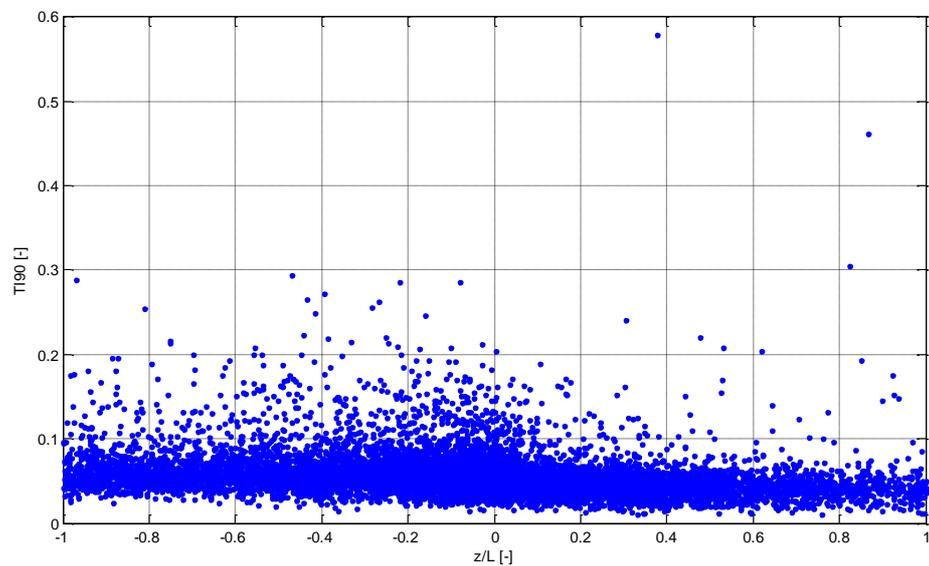
**Figure 19:** Correlation between turbulence intensity  $TI$  in 90 m height and stability parameter  $z/L$  at FINO 3 during year 2011.
