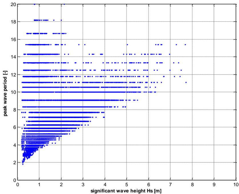
**Figure 30:** Correlation between significant wave height and peak wave period measured by the buoy at FINO 3 during year 2011.
