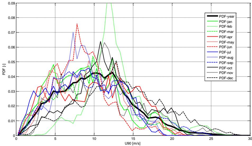
**Figure 13:** PDFs of the wind speed at FINO 3 in 90 m height for each month (thin lines) and for the whole year (thick line) of 2011.
