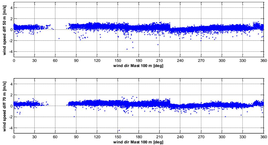
**Figure 9:** Corrected LiDAR measurements in 50 m (top) and 70 m (bottom) height at FINO 3 by blanking of the data in the mast shadow.
