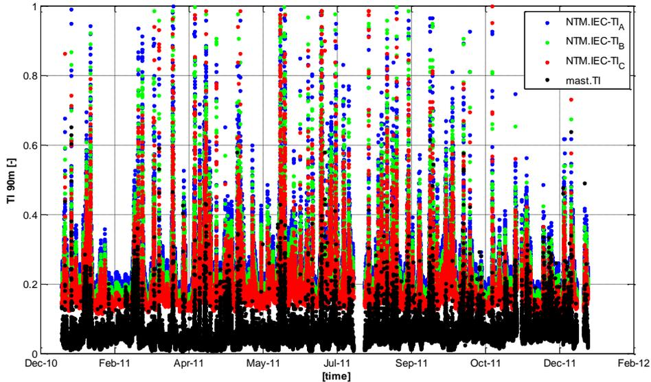
**Figure 21:** Turbulence intensity of the wind speed at FINO 3 in 90 m height and the theoretical values of the Normal Turbulence Model (IEC 61400-1 Ed.3) depending on the time of the year 2011.
