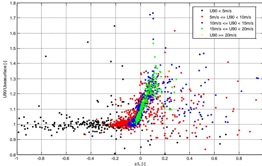
**Figure 17:** Stability parameter  $z/L$  at FINO 3 for 2011 depending on different wind shears  $U_{90}/U_{useasurface}$ .
