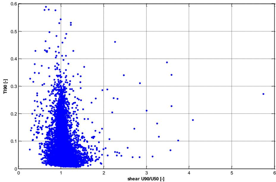
**Figure 18:** Correlation between turbulence intensity  $TI$  in 90 m height and wind shear  $U90/U50$  at FINO 3 during year 2011.
