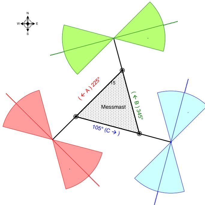
**Figure 7:** Illustration of undisturbed wind sectors, 2 x 60° for each of the booms A, B and C (source: GL GH).
