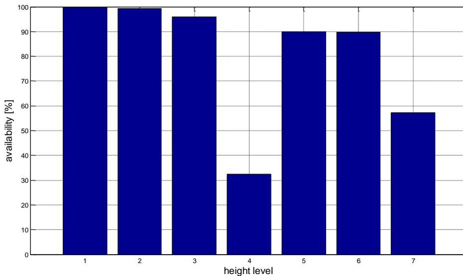
**Figure 23:** Availability of the LiDAR data at different height levels installed at FINO 3 from April to October of 2011.
