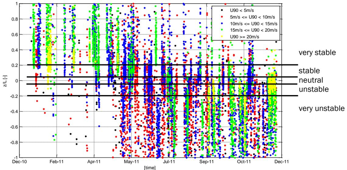
Figure 15: Stability parameter  $z/L$  at FINO 3 depending on the time of the year 2011.
