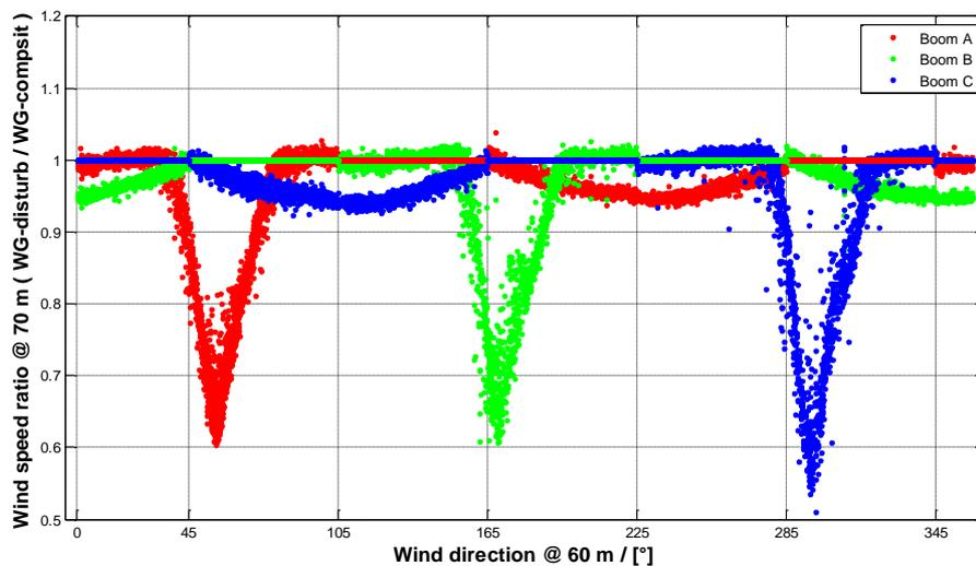
**Figure 6:** Mast effect on the anemometer measurements at 70 m height at FINO 3 (source: GL GH).
