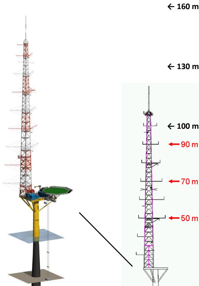
**Figure 5:** Design (left) and height details (right) of the cup anemometer (red) and the LiDAR (red + black) measurements at FINO 3.
