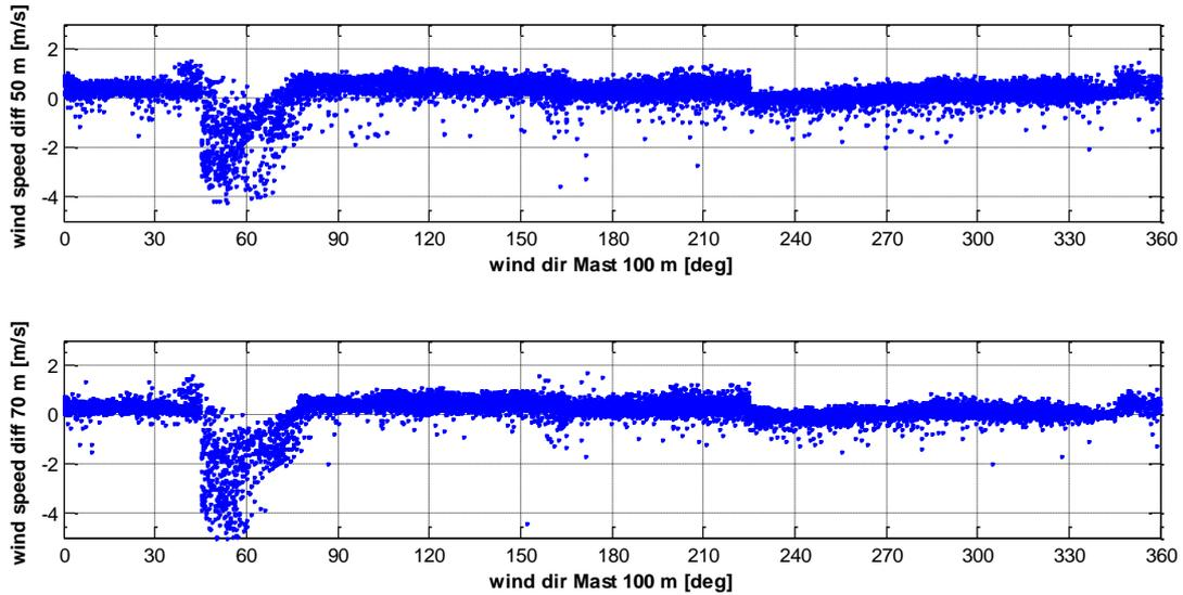
**Figure 8:** Mast effect of the met mast on the LiDAR measurements in 50 m (top) and 70 m (bottom) height at FINO 3.
