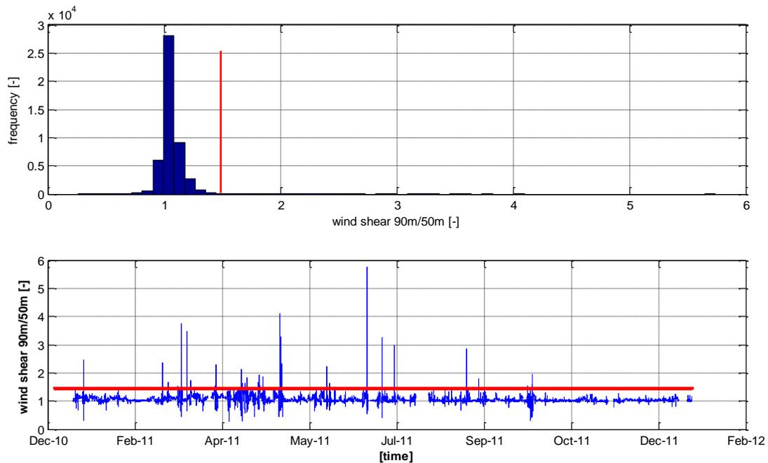
**Figure 34:** Frequency distribution and time series of the wind shear  $U_{90}/U_{50}$  at FINO 3 during year 2011, value of four times  $\sigma$  of shear marked with red line.
