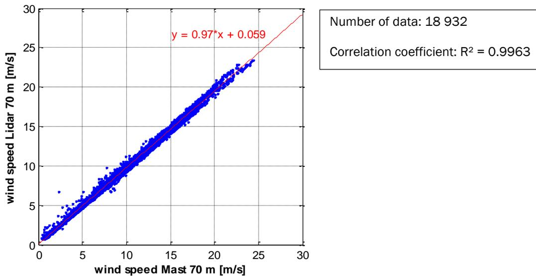
Figure 26: Correlation of the wind speed of the met mast and of the LiDAR at 70 m height at FINO 3.
