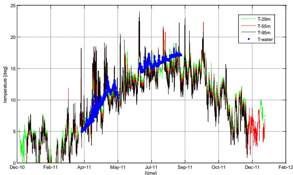
Figure 16: Temperature  $T$  in 29 m, 55 m and 95 m height at the met mast as well as the sea surface temperature at FINO 3 during year 2011.
