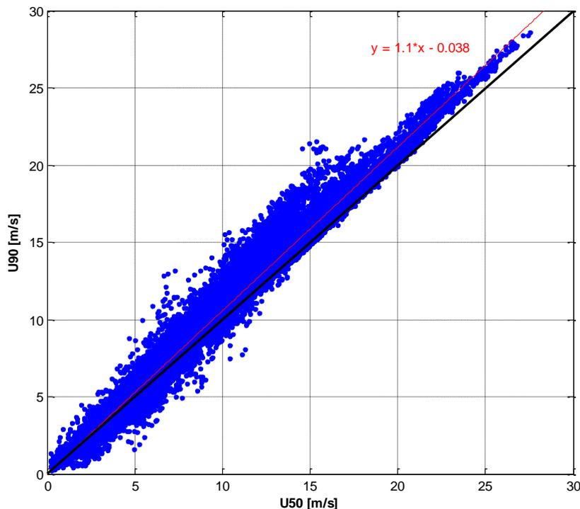
**Figure 33:** Scatterplot of the wind speeds in 50 m and 90 m height measured at the met mast on FINO3 during year 2011.
