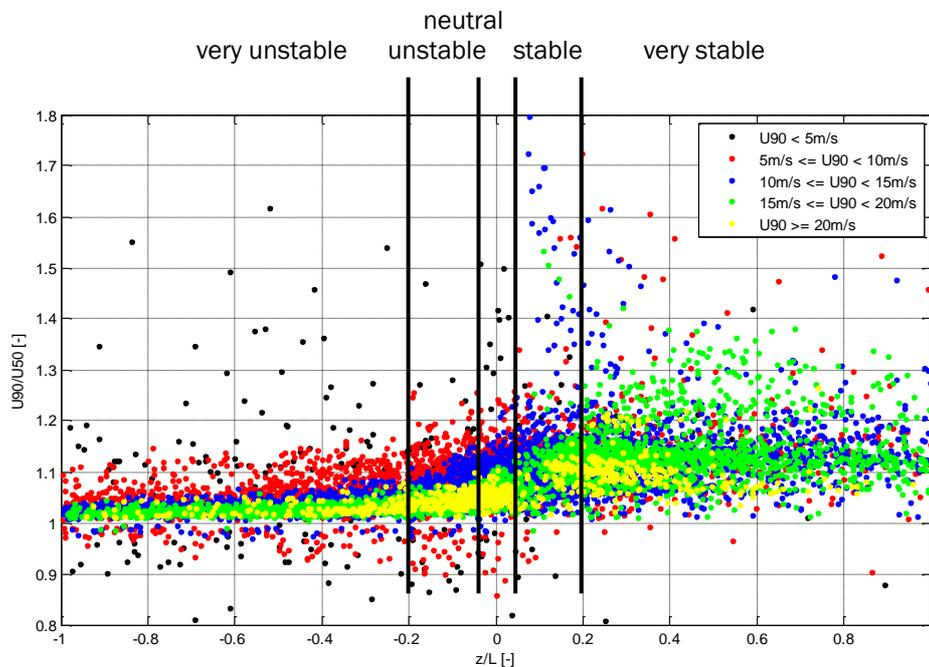
**Figure 14:** Stability parameter  $z/L$  at FINO 3 for 2011 depending on different wind shears  $U_{90}/U_{50}$ .
