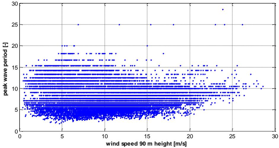
**Figure 29:** Correlation between peak wave period  $T_p$  and wind speed in 90 m height measured by the buoy at FINO 3 during year 2011.
