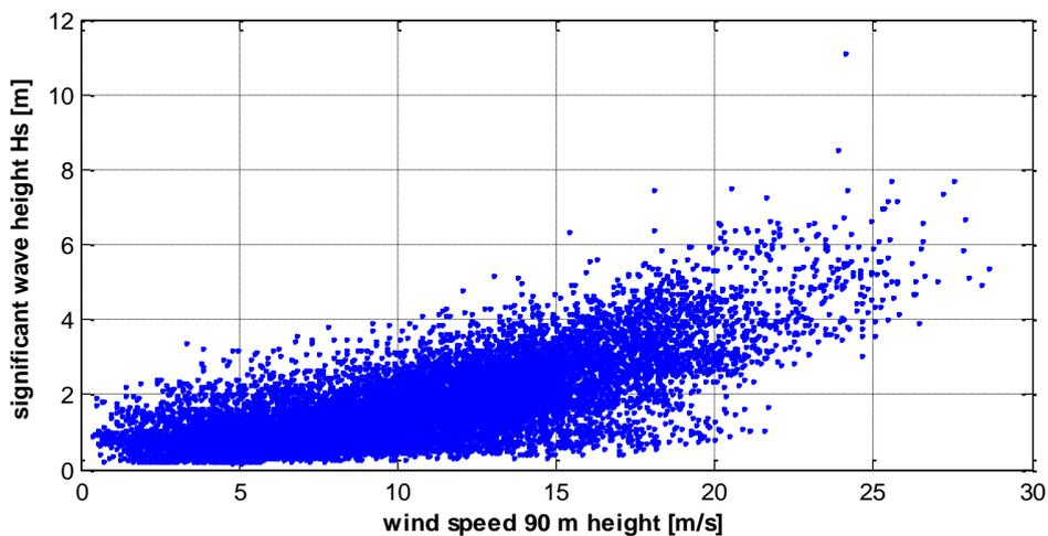
**Figure 28:** Correlation between significant wave height  $H_s$  and wind speed in 90 m height measured by the buoy at FINO 3 during year 2011.
