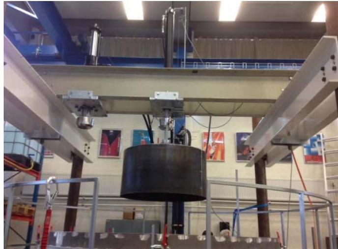
Figure 4.1-8: Bucket model of  $d/D=0.5$
