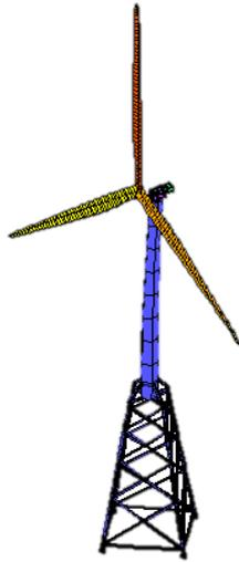
Figure 5.2-9: Tower mode 1 – side to side
