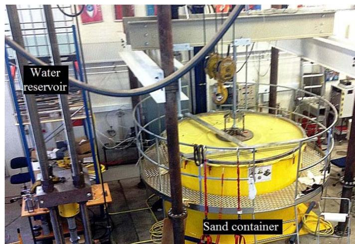
Figure 4.1-6: The test set-up of axially loaded bucket foundations
