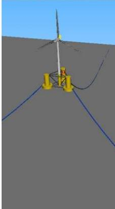
**Figure 3.12: SIMPACK OC4 model with dynamic mooring lines**
