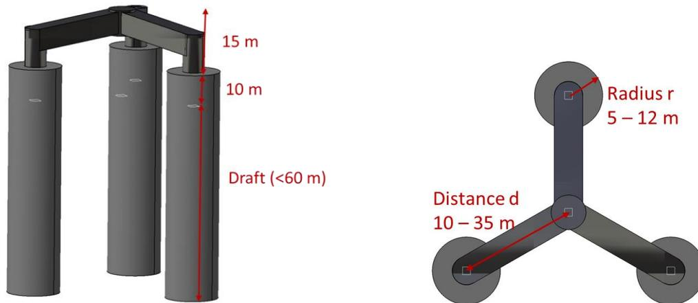
**Figure 3 - Platform geometry.**
