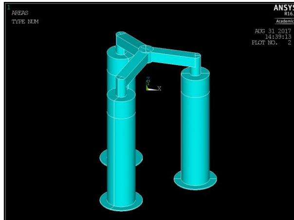
Figure 68: : model of the floating platform in ANSYS
