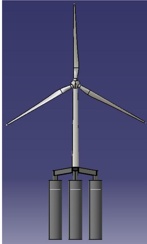
Figure 11 – INNWIND.EU TripleSpar platform with DTU10MW reference turbine.
