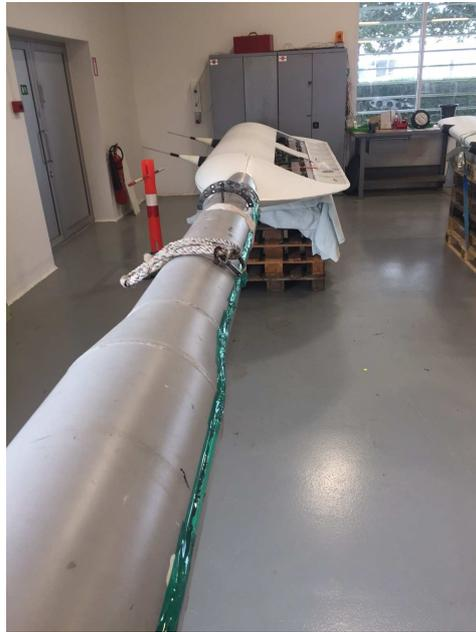
Figure 47 The morphing wing mounted on the rotating rig boom before installation.
