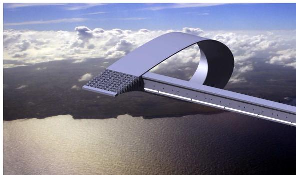
Figure 3. View of the turbine blade section with a morphing flap (Skins are removed for clarity purpose, Courtesy of DTU.)
