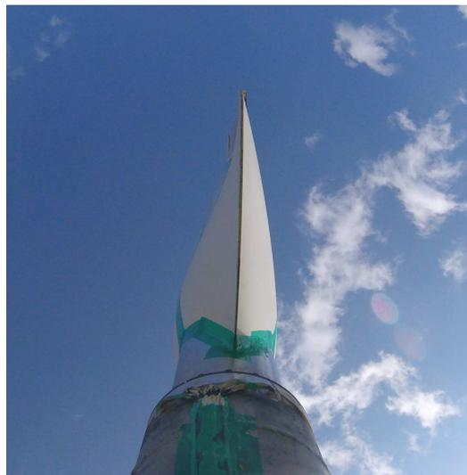
**Figure 122** Photo of wing with deflected flap during operation.
