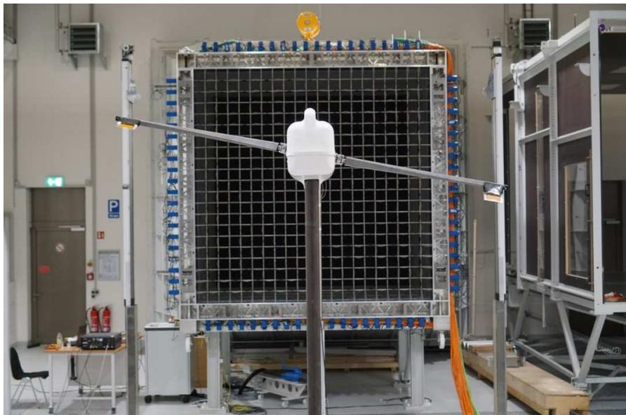
Figure 1, Wind tunnel experiments in Oldenburg with the active grid and a scaled innovative two-bladed wind turbine.
