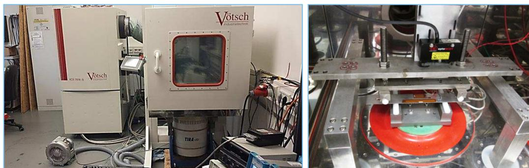
Figure 9: Four-point bending test set up
