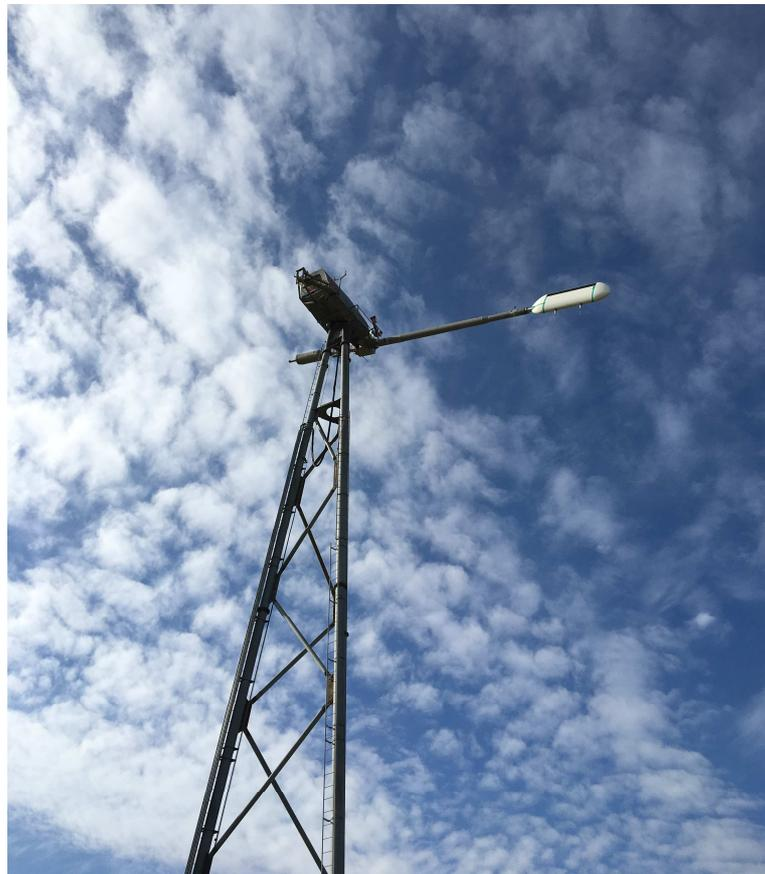
**Figure 46** The rotating rig with the mounted morphing wing.
