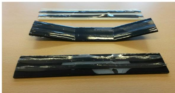
Figure 50, The grey rectangle on the top and the two black rectangles below it are the 3d printed samples post fracture, placed on a sandstone-coloured desktop that forms the background. Top: ABS M30, Middle: PC-ABS, Bottom: Nylon
