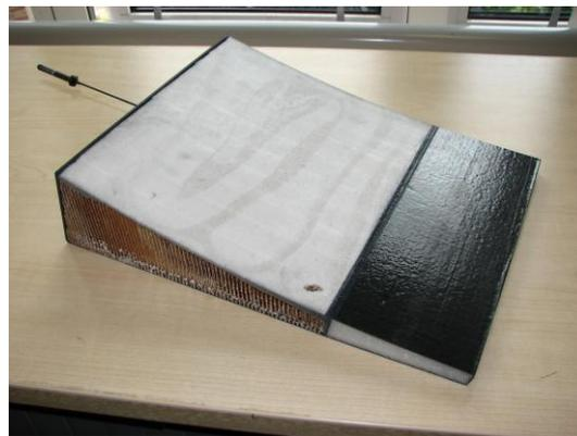
**Figure 91.** Morphing flap demonstrator seen with the pressure side upwards. For unknown reasons, bubbles gathered on the surface of the morphing skin at the time the foam was casted, resulting in a ~1cm<sup>2</sup> patch of uncovered honeycomb, as seen on the right hand bottom corner of the skin.
