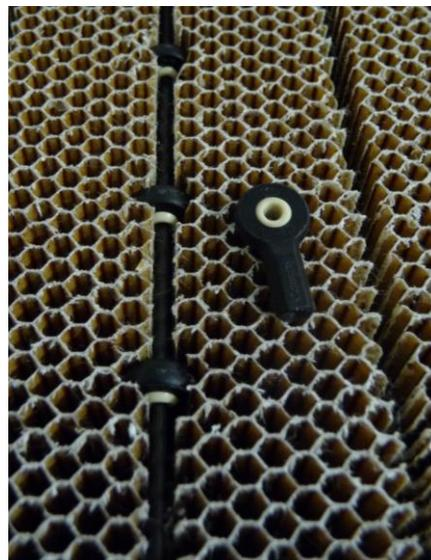
**Figure 90. Photograph detailing the rod ends inserted in the honeycomb core before the foam skin is applied.**
