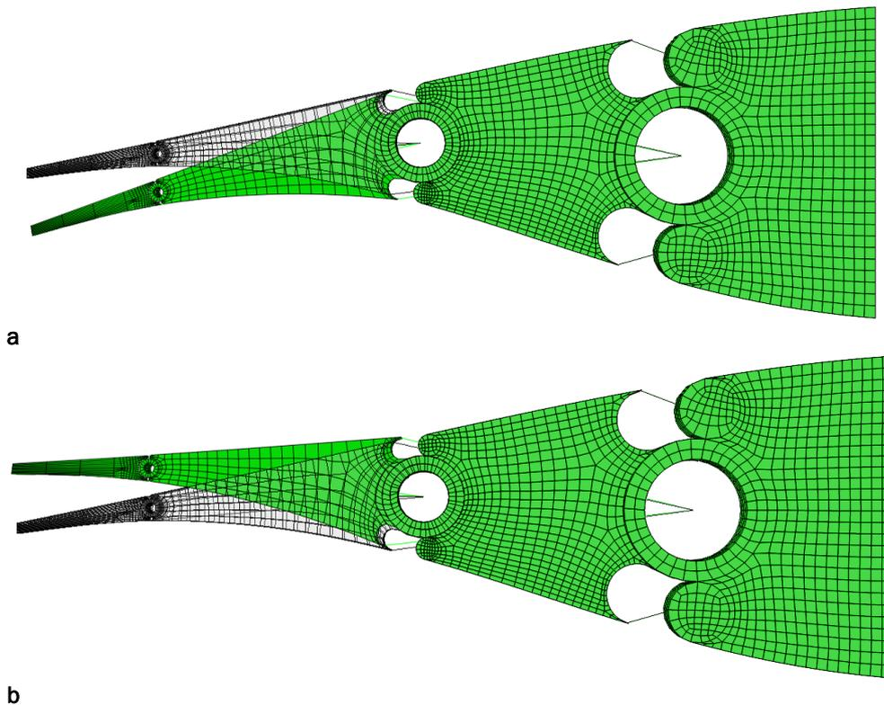
Figure 44: Morphing mechanism at 30% of chord length activated for (a) downwards and (b) upwards movement
