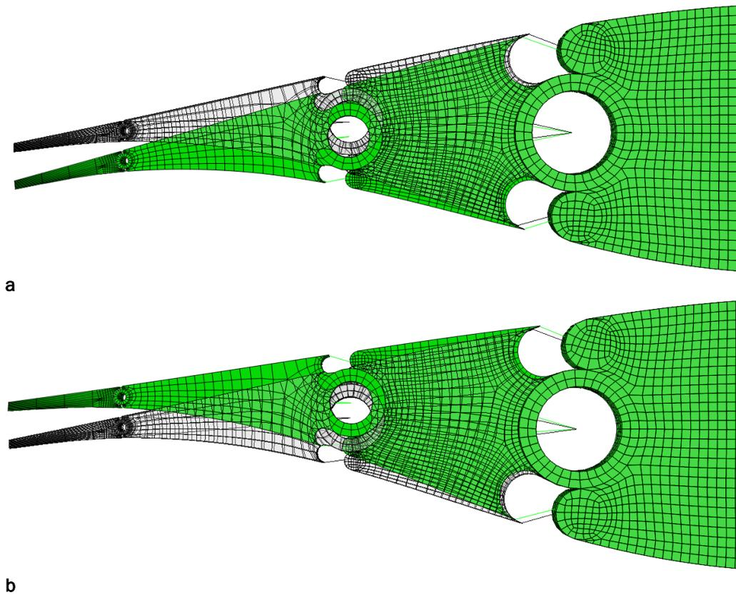
Figure 50: Morphing Mechanism at 50% of chord length activated for (a) downwards and (b) upwards movement
