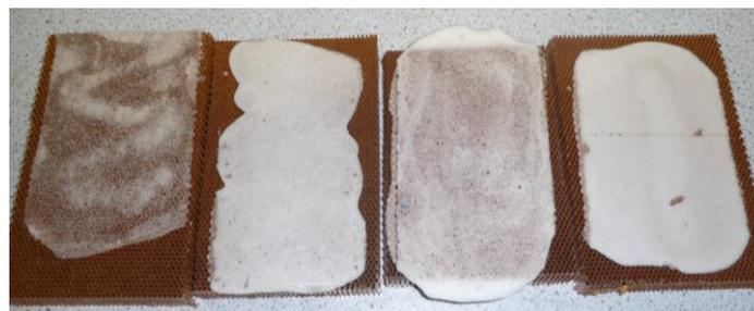
**Figure 81. Photographs of different morphing skin samples. One can notice the increasing quality of the surface of the foam. From left to right: 2:1 polyol to isocyanate mixing ratio / no release agent; 2:1.5 polyol to isocyanate mixing ratio / no release agent; 2:1.125 polyol to isocyanate mixing ratio / silicon release agent; 2:1.125 polyol to isocyanate mixing ratio / wax release agent.**
