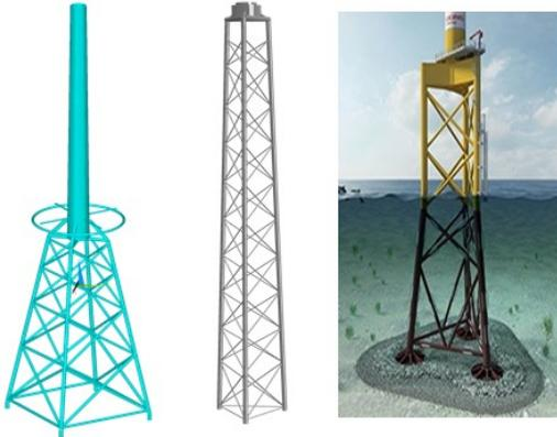
Three legged frame structures, also as a full length structure to the nacelle or for legged structures with vibration absorption devices
