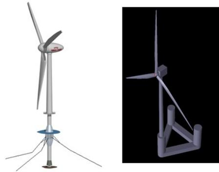
Guyed Tower with buoyancy and ballast chambers and Semi Submersible designed for a 10 MW wind turbine.
