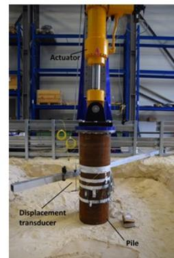
Tensile static test of Pile 2
