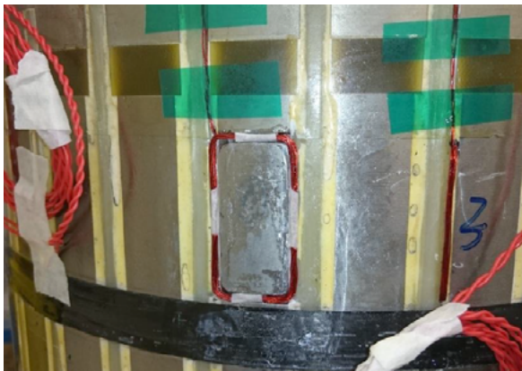
FIGURE 4.29 Insertion of search coils on pole-piece rotor
