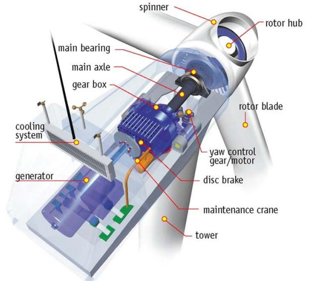
Fig. 3. Sketch of a nacelle with gearbox, in this case of a constant speed NEG micon wind turbine. Source: Bundesverband WindEnergie e.V.
