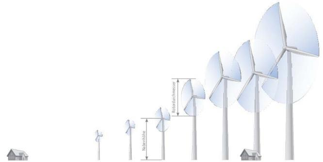
Fig. 1. Development of power and size of wind turbines. Source: Bundesverband WindEnergie e.V.
