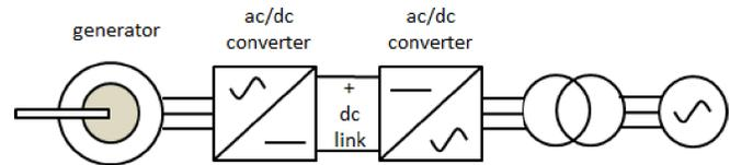
Fig. 15. Overview of the power conversion components.
