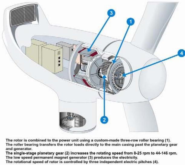
Fig. 4. Sketch of the multibrid system. Source: Winwind.
