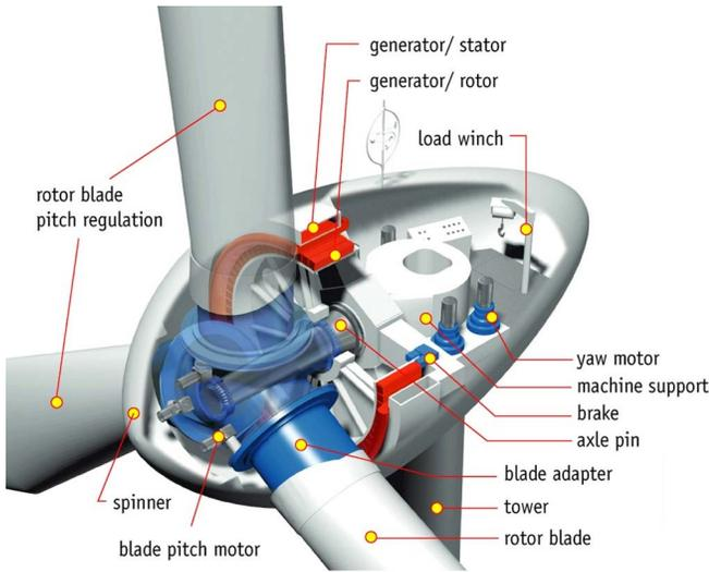
Fig. 5. Sketch of a gearless nacelle, in this case of an Enercon E-66 DD wind turbine. Source: Bundesverband WindEnergie e.V.
