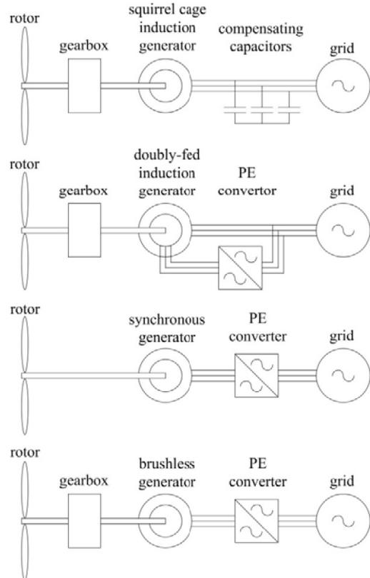
Fig. 2. Four commonly used generator systems [18].
