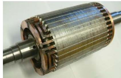
Fig. 7. Rotor of a brushless DFIG with six nested loops, as used in a machine with a stator with a four-pole and an eight-pole winding.
