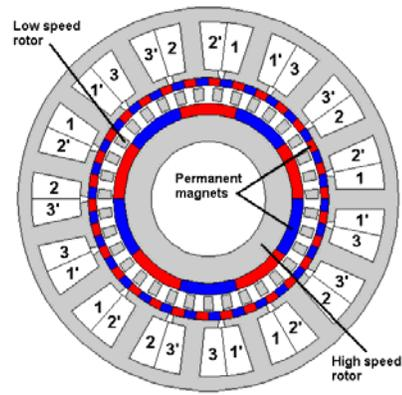
Fig. 9. PDD with magnetically and mechanically coupled magnetic gear and electrical machine.
