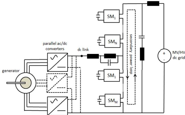
Fig. 18. Transformerless modular multilevel converter with dc link [98].
