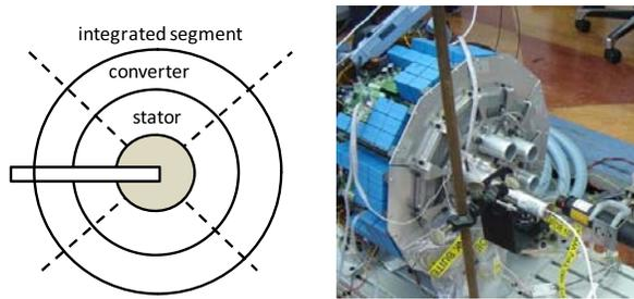
Fig. 17. Segmented fault tolerant generator-converter system.
