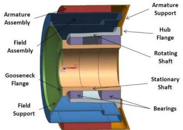
Fig. 12. Proposed 10-MW LTS wind turbine generator from GE. Reproduced from [78].
