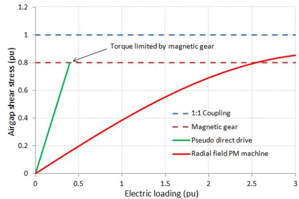
Fig. 10. Air-gap shear stress in PDD and radial field PM machines (electric loading of 1 pu corresponds to the thermal limit of a radial field PM machine).
