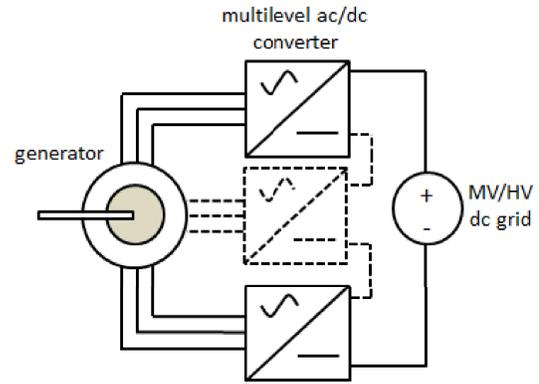
Fig. 16. Generator-converter modular multilevel system.
