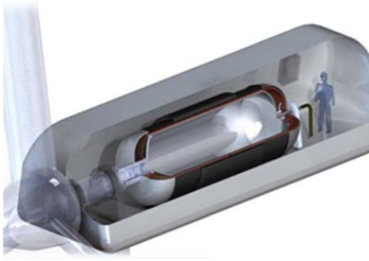
Fig. 14. Proposed 10-MW MgB<sub>2</sub> wind turbine generator from AML. Reproduced from [81].
