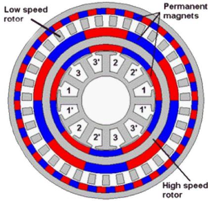
Fig. 8. Electrical machine accommodated in the bore of high-speed rotor of magnetic gear.
