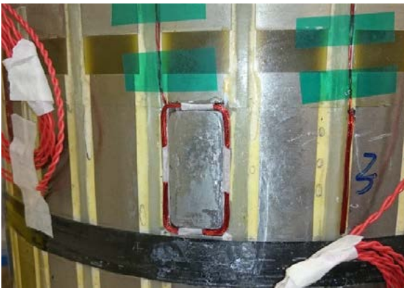
FIGURE 4.29 Insertion of search coils on pole-piece rotor
