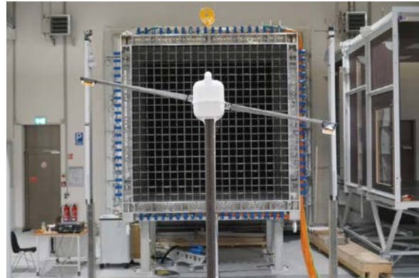
FIGURE 4.11 Wind tunnel experiments in Oldenburg with the active grid and an scaled innovative two-bladed wind turbine
