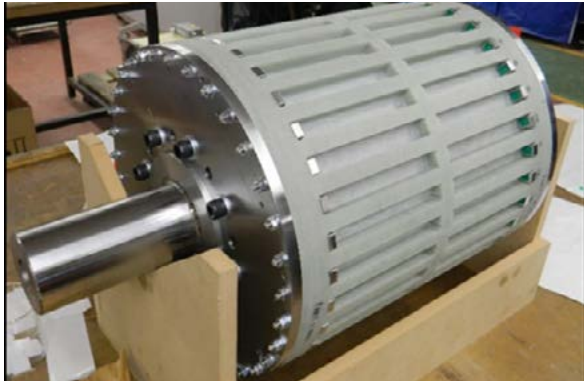
FIGURE 4.31 Monocoque pole-piece rotor structure for 5 kNm prior to insertion of pole-pieces
