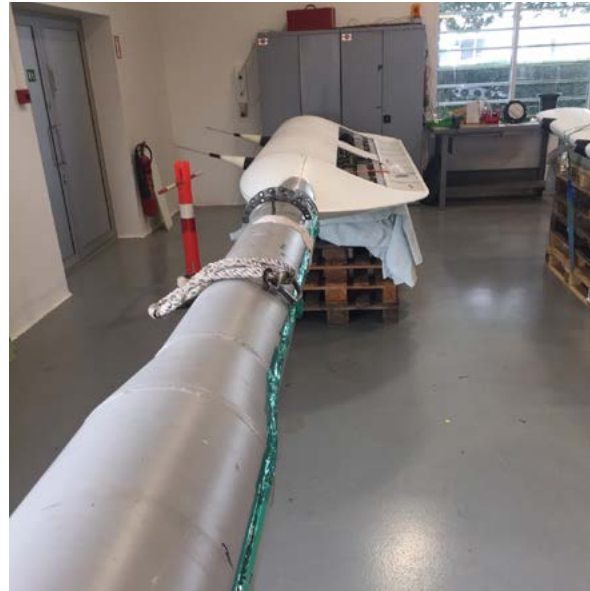
FIGURE 4.16 A new 2 m blade section has been manufactured for the INNWIND.EU flap testing on the rotating test rig.
