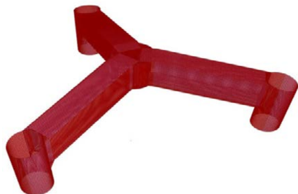
FIGURE 4.48 Structural mesh for the Finite Element analysis of the transition tripod
