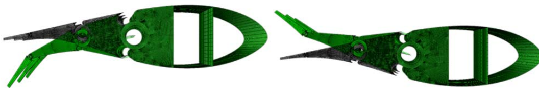
Figure 44: Morphing capabilities by applying a modular flap controlled by SMAs.
