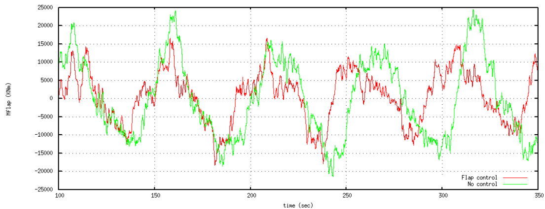
Figure 78: Time series of the flapwise bending moment at the blade root at standstill. Wind speed 42.5m/s, yaw 15°.
