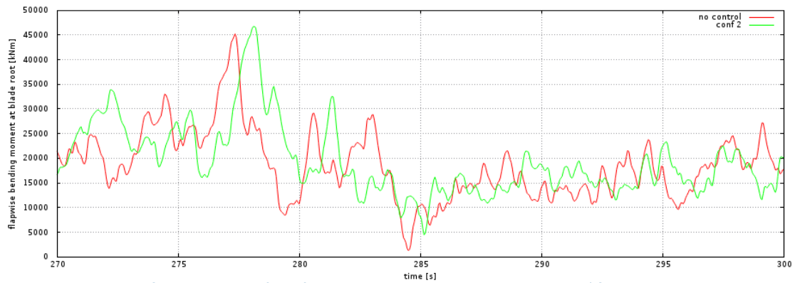
Figure 73: Time series of the flapwise bending moment. Wind speed 16m/s, R5, ETM.
