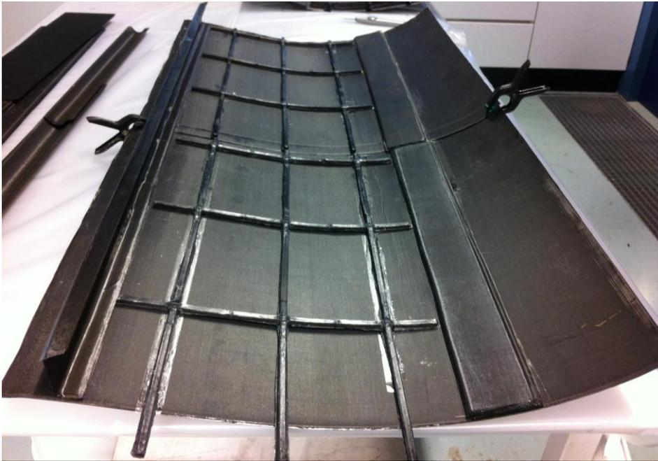
Figure 128: Skins placed edge to edge and held together by clamps. Grids are glued to the skins
