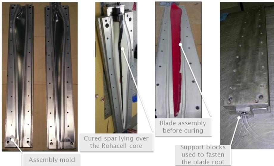
**Figure 9** Blade sub-components assembly.
