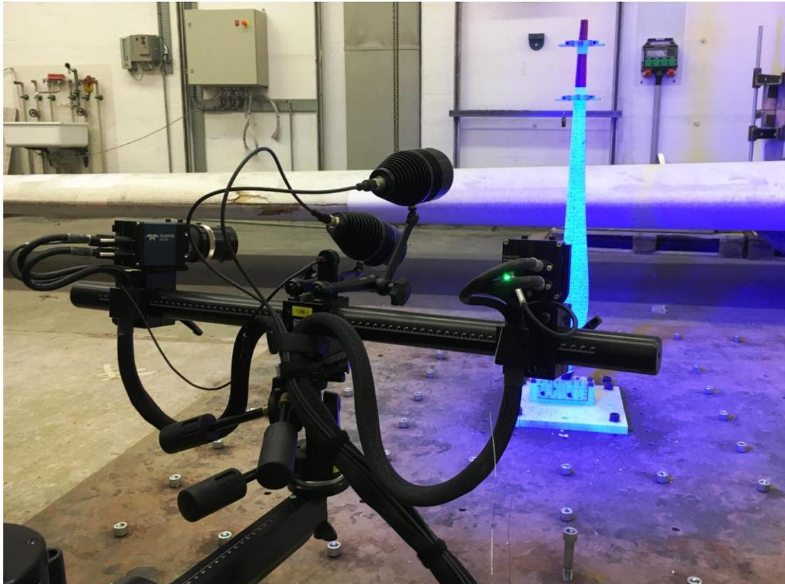
Figure 39 Static blade test setup with DIC camera boom in front.
