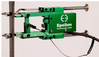
**Figure 148:** Epsilon Axial Extensometer
