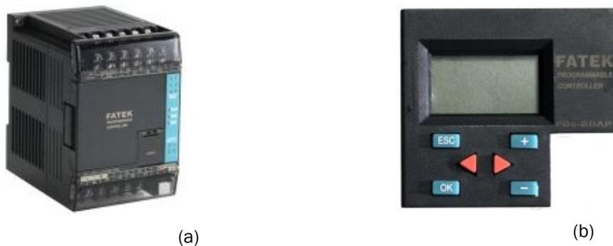
**Figure 141:** The Programmable Controller (a) unit and (b) the LCD screen.
