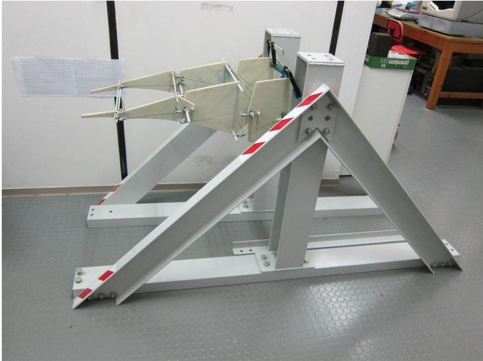
**Figure 87:** Morphing section prototype mounted on the test rig
