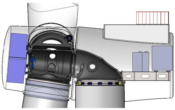
The PDD generator is more compact than the SCDD generator design and is easy to integrate within the rotor spinner cover.
