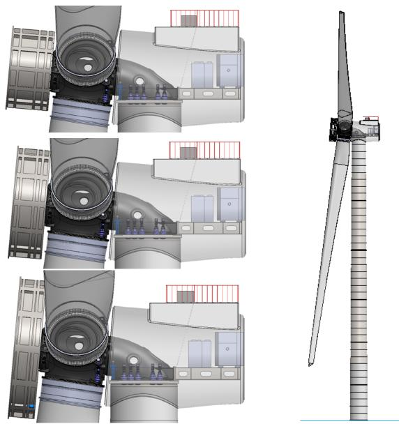
For all three generator configurations there is clearance between the generator structure and blade although for SCDD3 the clearance is small.
