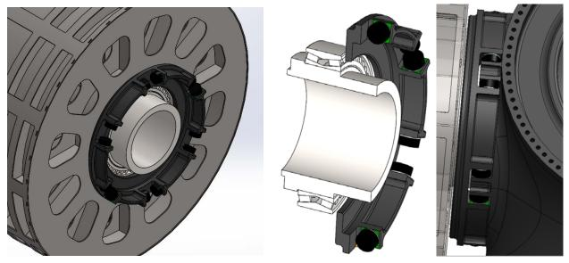
The hydraulic pads transmit the torque by the stiff behaviour in the pad normal direction but the pads are compliant in the other directions isolating the generator from the relative deflections between the rotor hub and kingpin.
