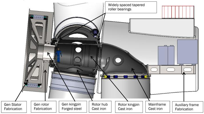
Figure 3-9: Cross section Concept 1-SCDD, SCDD2 example
