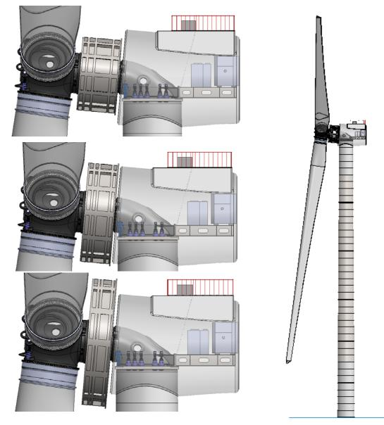
For all three configurations there is sufficient clearance between the generator and blades due to the blade cone angle and there is also enough space between the generator and the tower because of the drivetrain tilt angle.
