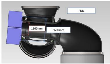
Figure 3-1: Figure 3.5 from [3]: Main PDD interface dimensions
