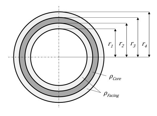
Fig. 3: Cross-section of sandwich tube with corresponding quantities
