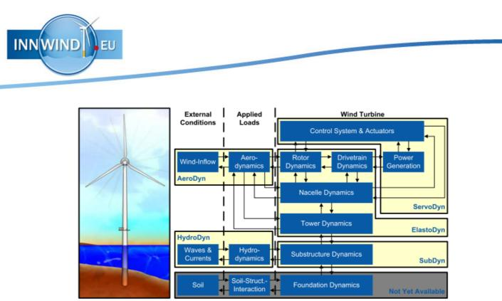
Fig. 2: Modular structure of aero-hydro-servo-elastic simulation framework FAST [18]
