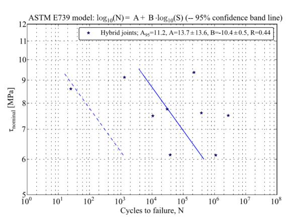
Fig. 6: Experimental S-N curve for hybrid joints
