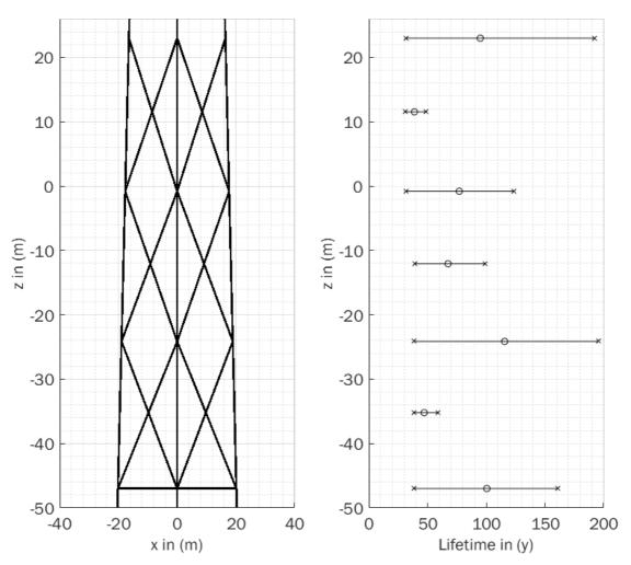
Fig. 10: Hybrid joint lifetimes of ideal jacket for each joint layer. Crosses show the minimum and maximum lifetimes on each layer, circles the corresponding mean lifetime.
