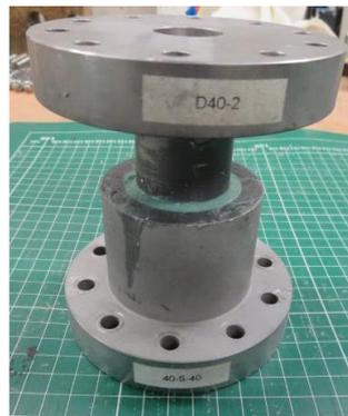
Figure 10: single overlap small-scale tension, torsion and mixed mode specimens [3-09]
