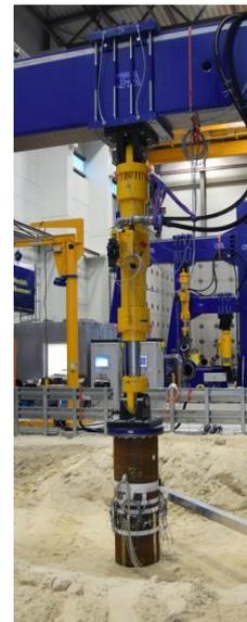
**Figure 17: Tensile testing of Pile 2. Test campaign of Fraunhofer IWES at the test centre for support structure in Hannover (Testzentrum Tragstrukturen Hannover, TTH), 2015.**
