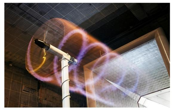
Figure 2-5: The 5m MEXICO model rotor installed in the DNW 9.5x5m wind tunnel late June 2014
