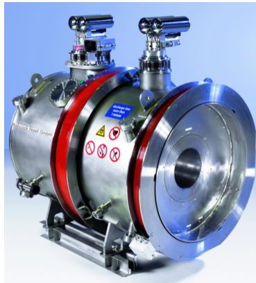
Figure 2.21: Cylindrical cryostat of a commercial product (Babcock Noell GmbH). [95]
