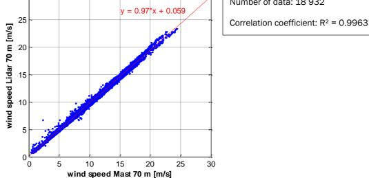
Figure 26: Correlation of the wind speed of the met mast and of the LiDAR at 70 m height at FINO 3.
