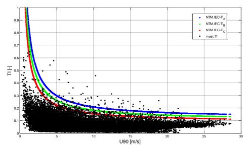
**Figure 20:** Turbulence intensity TI of the wind speed at FINO 3 in 90 m height and the theoretical values of the Normal Turbulence Model (IEC 61400-1 Ed.3).
