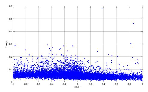
Figure 19: Correlation between turbulence intensity TI in 90 m height and stability parameter z/L at FINO 3 during year 2011.
