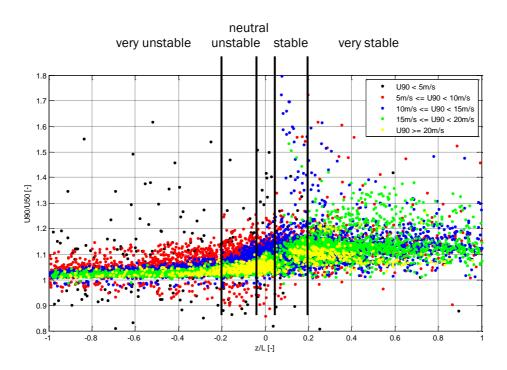
Figure 14: Stability parameter z/L at FINO 3 for 2011 depending on different wind shears U90/U50.
