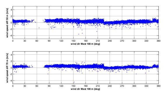
Figure 9: Corrected LiDAR measurements in 50 m (top) and 70 m (bottom) height at FINO 3 by blanking of the data in the mast shadow.
