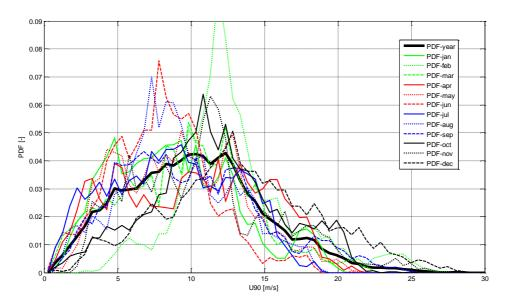
Figure 13: PDFs of the wind speed at FINO 3 in 90 m height for each month (thin lines) and for the whole year (thick line) of 2011.
