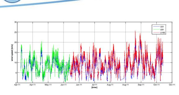
Figure 24: Time series of the LiDAR data in 51 m, 71 m and 91 m height at FINO 3.
