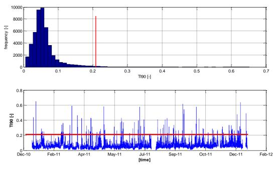
**Figure 31:** Frequency distribution and time series of the turbulence intensity TI at FINO 3 during year 2011, value of four times  $\sigma$  of TI marked with red line.
