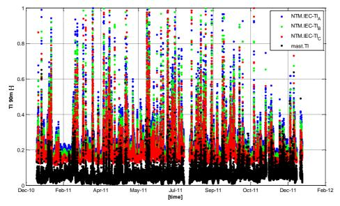
**Figure 21:** Turbulence intensity of the wind speed at FINO 3 in 90 m height and the theoretical values of the Normal Turbulence Model (IEC 61400-1 Ed.3) depending on the time of the year 2011.
