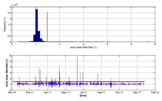
**Figure 34:** Frequency distribution and time series of the wind shear U90/U50 at FINO 3 during year 2011, value of four times  $\sigma$  of shear marked with red line.
