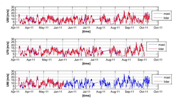
**Figure 25:** Comparison of the time series of the LiDAR data with mast data in 50 m (top), 70 m (middle) and 90 m (bottom) height at FINO 3.
