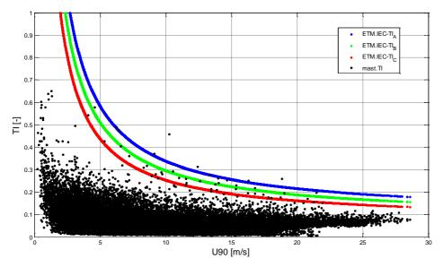
**Figure 22:** Turbulence intensity TI of the wind speed at FINO 3 in 90 m height and the theoretical values of the Extreme Turbulence Model (IEC 61400-1 Ed.3).
