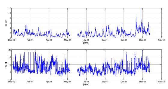
Figure 27: Time series of the significant wave height Hs (top) and the peak wave period Tp (bottom) measured by the buoy at FINO 3 during year 2011.
