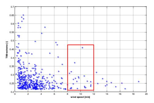
Figure 32: Extreme turbulence intensities in dependence to the wind speed at FINO 3, exemplary wind condition 1 marked with red box.
