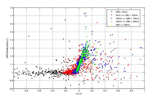
Figure 17: Stability parameter z/L at FINO 3 for 2011 depending on different wind shears U90/Useasurface.
