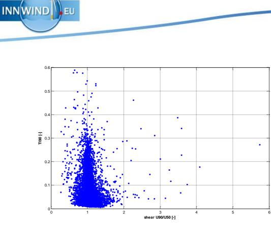
Figure 18: Correlation between turbulence intensity TI in 90 m height and wind shear U90/U50 at FIN0 3 during year 2011.
