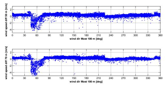
Figure 8: Mast effect of the met mast on the LiDAR measurements in 50 m (top) and 70 m (bottom) height at FINO 3.
