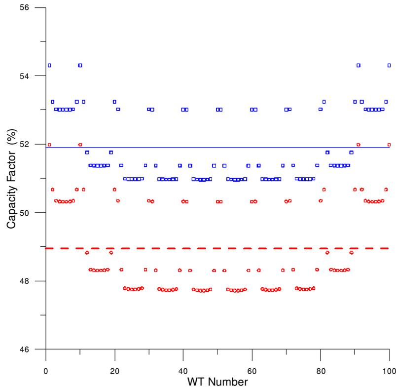
Figure 4 **Capacity factor and wake losses per turbine in a 10X10 offshore wind farm with 5 MW turbines at 8D spacing. Red dots refer to the initial turbines (“standard”, highly loaded) and blue squares to the less loaded (“low-induction”) turbines. The dashed red and the blue line correspond to the wind farm mean values.**
