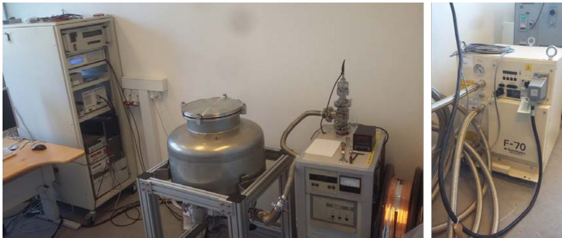
Figure 8-6 Cryostat with turbo pump for establishing the vacuum and electronics for measuring the properties of the superconducting MgB 2 test coil. The cold head sitting in the cryostat is connected to the F-70 helium compressor placed in the room behind the wall ( picture to the right).
