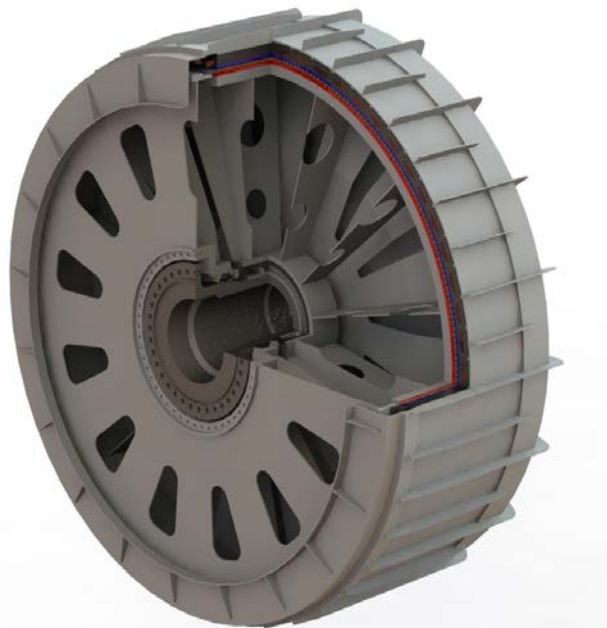
Figure 3-3 – 20MW Magnetic PDD generator that is designed for front-mounted operation. The torque-only coupling allows bearings to be sized based on the generators own static and dynamic loads. The king-pin type design reacts main torque through the central stub-shaft of the PDD.
