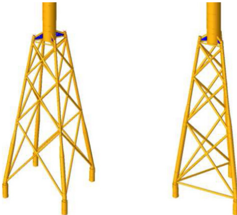
Figure 4-8: Schematic of 3 and 4 legged jacket type sub structures
