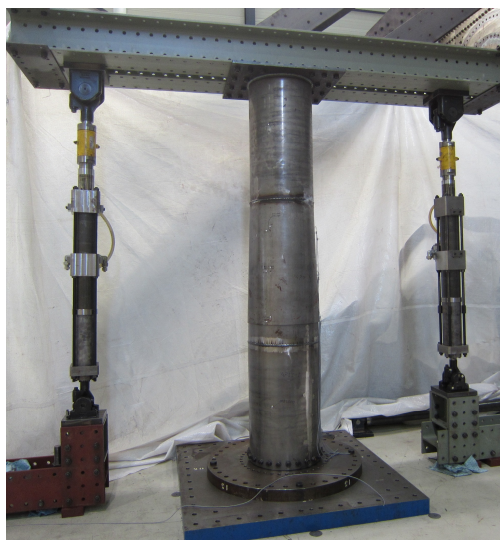
Figure 3-10: Experimental set-up from the FLOW slip joint project
