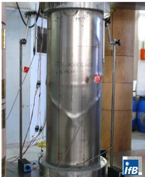
Figure 3-7: Sandwich structure with UHPC core under ultimate loads acc. to Lindschulte [LUH05]
