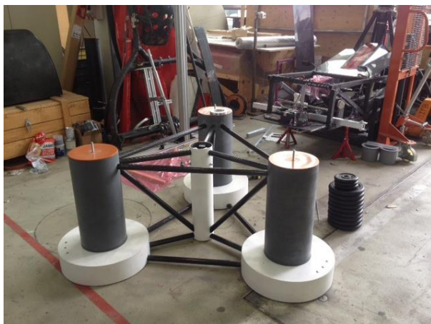
Figure 2-7 Scaled OC4-DeepCWind model at the University of Stuttgart (left) and model description by (Robertson A. , et al.) (right).
