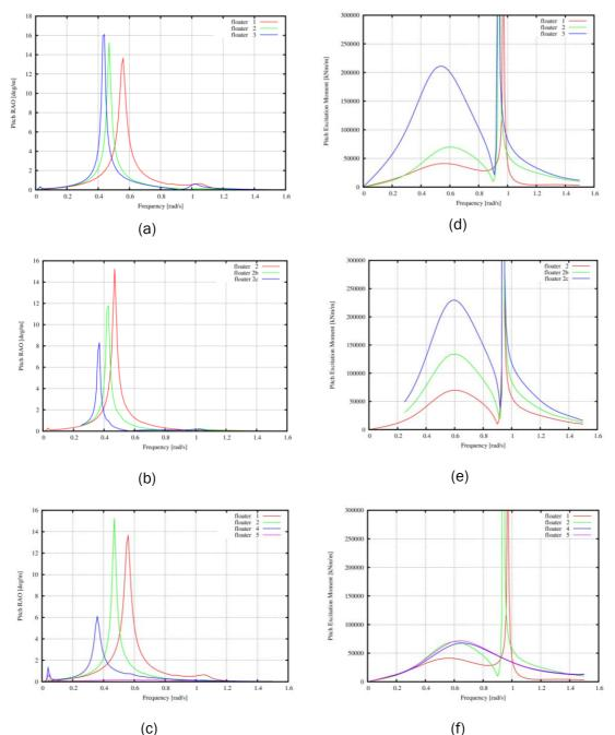
Figure IV.6 – RAOs (Left column) & Excitation Moment plots (right column) in pitch. Figures (a,d) show dependence on the draft (ID1=10m, ID2=20m, ID3=30m). Figures (b,e) show the influence of heave plates on the ID2 floater for the same draft of 20m. Figures (c,f) compare floaters of different dimensioning without heave plates for drafts of 10m (ID1 and 5) and 20m (ID 2,4).
