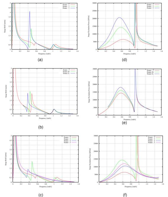
Figure IV.5 – RAOs (Left column) & Excitation Force plots (right column) in surge. Figures (a,d) show dependency on the draft for floaters with the same inner and outer diameters, Figures (b,e) show the effect of adding heave plates on the ID2 floater, and Figures (c,f) compare floaters of different dimensioning without heave plates for drafts of 10m (ID1 and 5) and 20m (ID 2,4).
