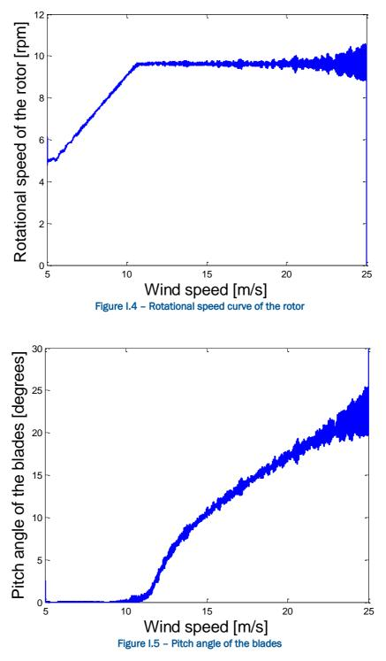
The values obtained in Figure I.2 to Figure I.5 show that the power curve of the 10MW turbine is maintained and that at high mean wind speeds, there is some oscillations of the thrust force due to the pitching of the platform. The influence of the significant wave height has been found minimal in these results.
