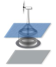
Figure II.3 – USTUTT spar: Conceptual Sketch.
