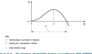
Figure 0.1 – Illustration of stability terms according to ISO 19901-6
