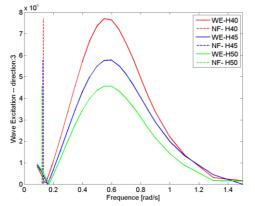
Figure II.12 – USTUTT spar: Translational normalized wave excitation response in heave (VarDraft).
