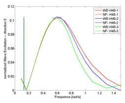
Figure II.13 – USTUTT spar: Translational normalized wave excitation response in heave (VarCost).
