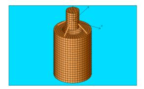
Figure II.6 – USTUTT spar: Example geometry as Ansys model.
