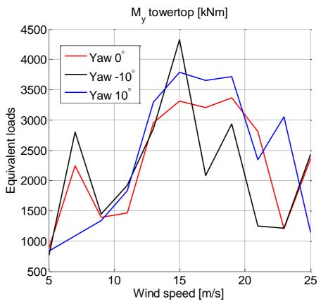
Figure I.8 – Equivalent Tower Top side-side fatigue moment for the lifetime of the turbine
