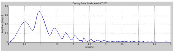
Figure III.6 – Surge excitation force divided by total floating offshore wind turbine mass
