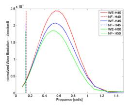
Figure II.10 – USTUTT spar: Rotational normalized wave excitation response in pitch (VarDraft).
