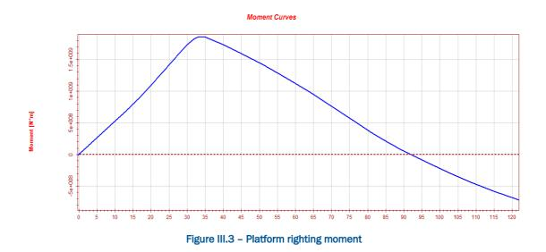
The righting moment increases with the inclination angle until it reaches a maximum close to 2.0-10<sup>8</sup> Nm around 34deg. For higher values of inclination, the righting moment decreases until 92 deg, where the platform would capsize. For an inclination angle of 3.5 deg the righting moment equals the maximum heeling moment (1.785-10<sup>8</sup> Nm) produced by the rotor thrust at the rated wind speed, which is consistent with the design conditions defined in [34].
