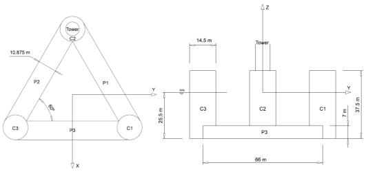
Figure III.2 - Plan (left) and Side (right) view of the platform
