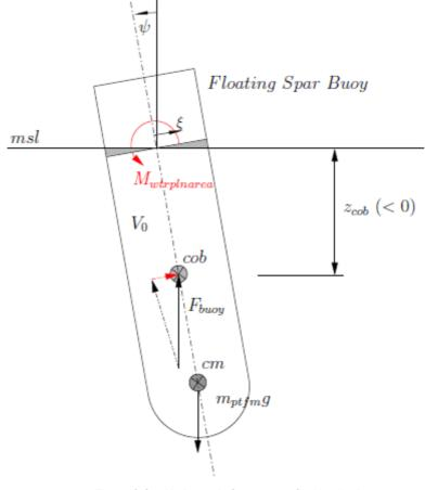
Figure 0.3 – Hydrostatic forces on a floating body
