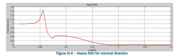
The plot shows that for very low values of angular frequencies (until 0.13 rad/s) the heave response is 1 meter, because the wave length is higher than the platform dimensions. The maximum response appears at a wave frequency close to the heave natural frequency. Finally, for high wave frequencies (higher than 1 rad/s) the platform response in heave is low.
