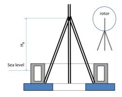
Figure IV.2 – A mixed buoyancy-ballast floater (Concept 1)
