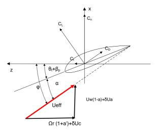
Figure IV.4 – Definition of the aerodynamic set-up
