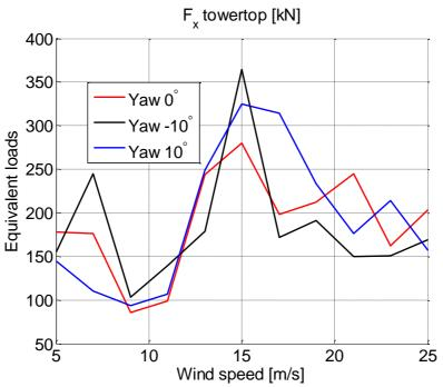
Figure I.6 – Equivalent Tower top Side Side fatigue force for the lifetime of the turbine
