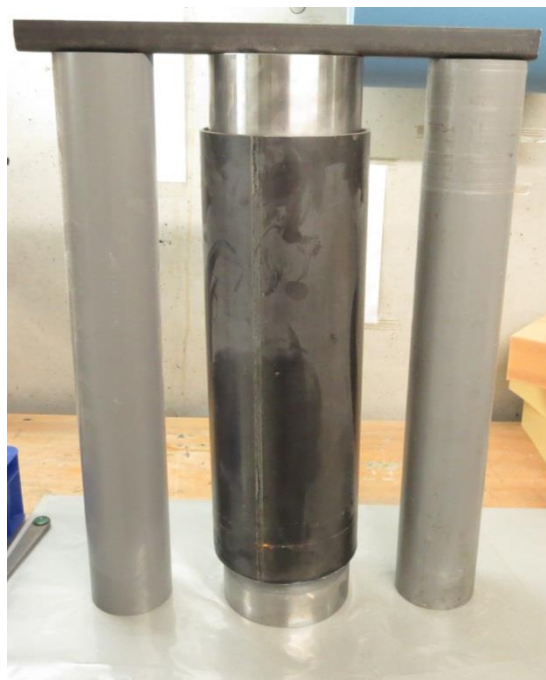
Figure 3.2-9 – Coupon bonded on both sides.
