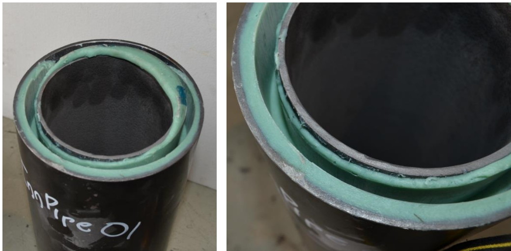
Figure 3.2-13 – Test joint subcomponent coupons InnPipe01 failure details.
