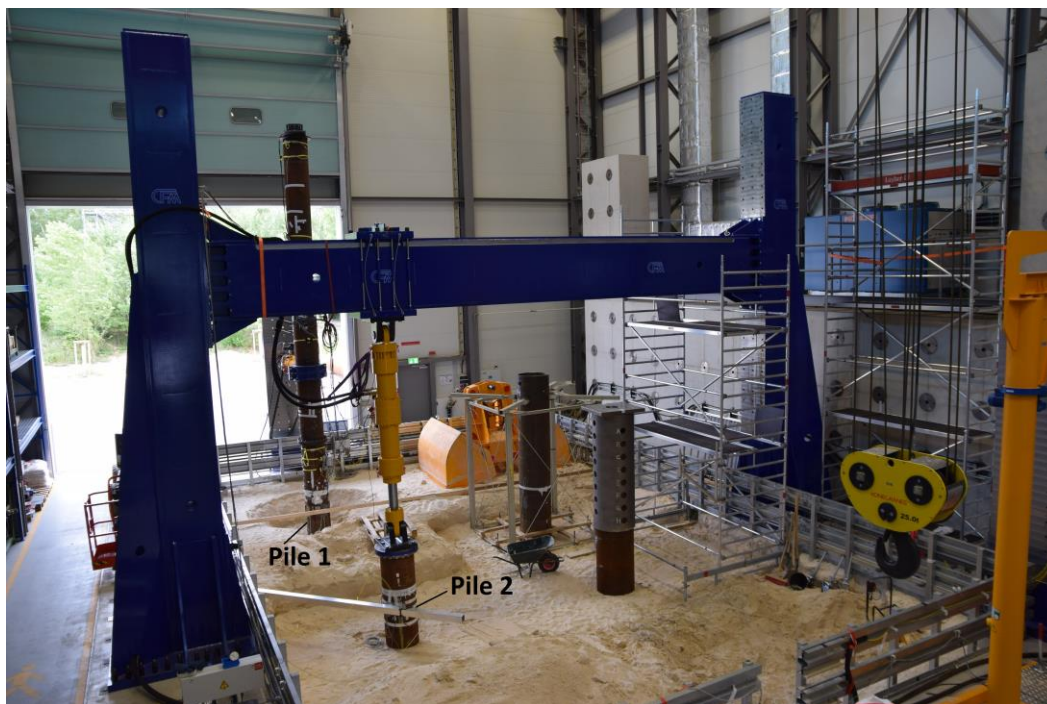
Figure 4.2-14 – Picture of the test setup just before the tensile loading test of Pile 2. Both piles for the INN WIND.EU project are depicted.
