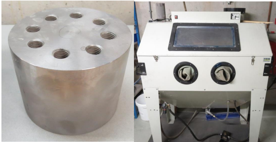
Figure 3.2-8 – Transition part sandblasted (left). Sand blasting machine (right).
