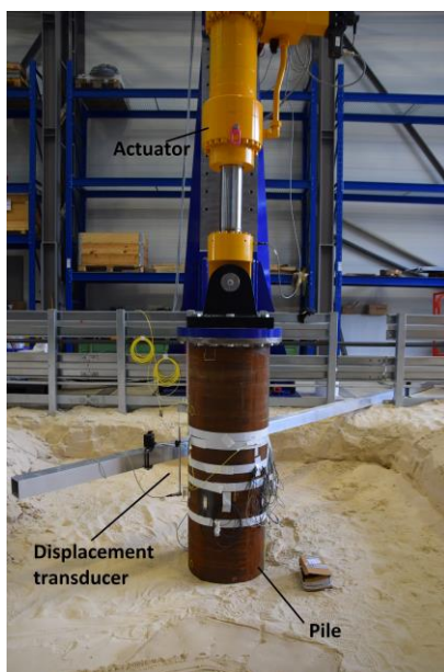
Figure 4.2-18– Pile 2 before the tensile loading test.
