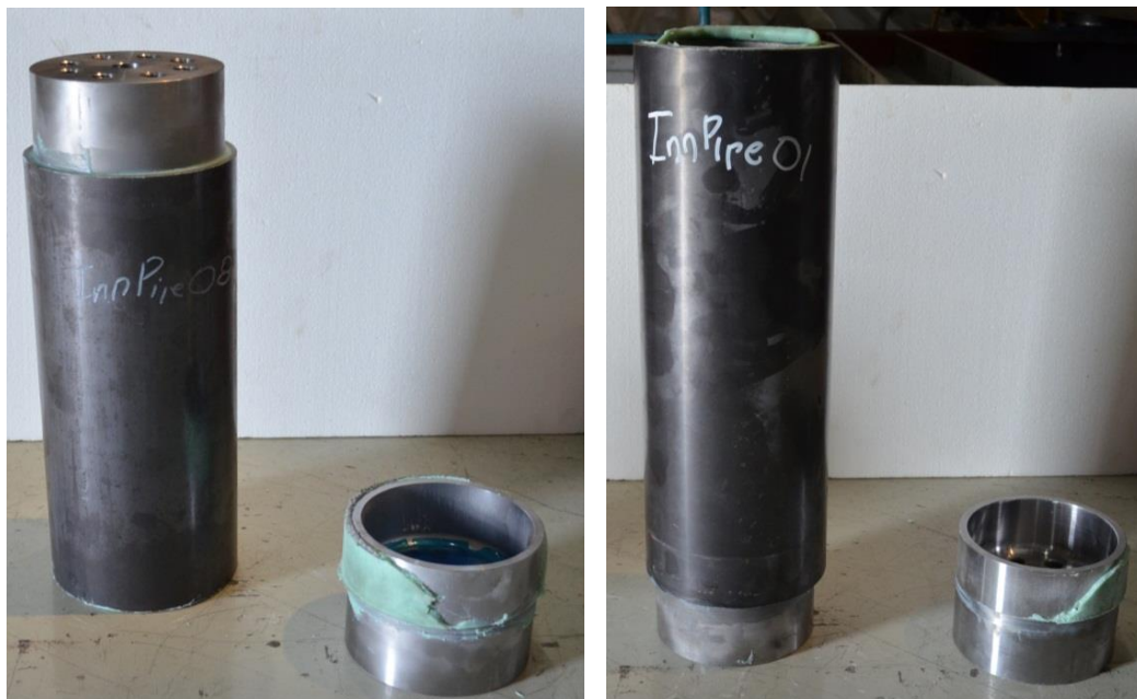
Figure 3.2-12 – Test joint subcomponent coupons InnPipe01 and InnPipe08 after static test.
