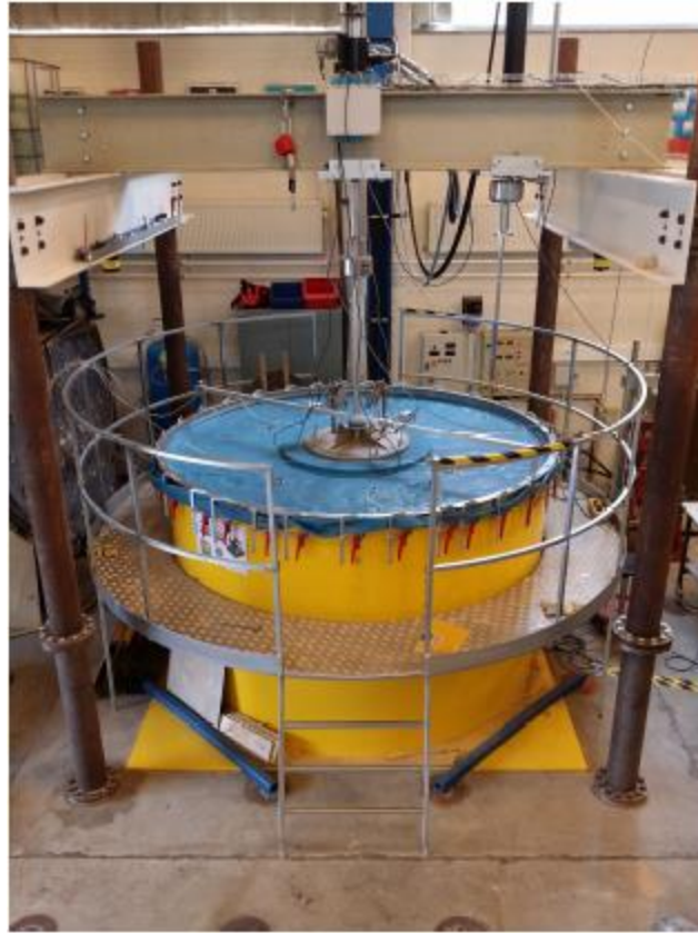
Figure 4.1-2 – Loading rig with installed bucket foundation and applied overburden pressure on the soil surface.
