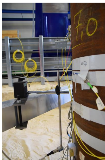
Figure 4.2-19– Particular of Pile 2 setup, displacement transducer.
