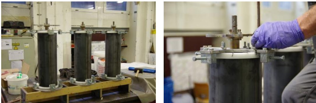
Figure 3.1-2 – Specimen preparation – concentrically aligned steel tubes (left) and filling of core material (right).
