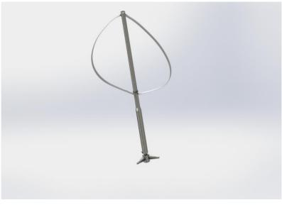
Figure 50 : SolidWorks rendering of the DeepWind concept
