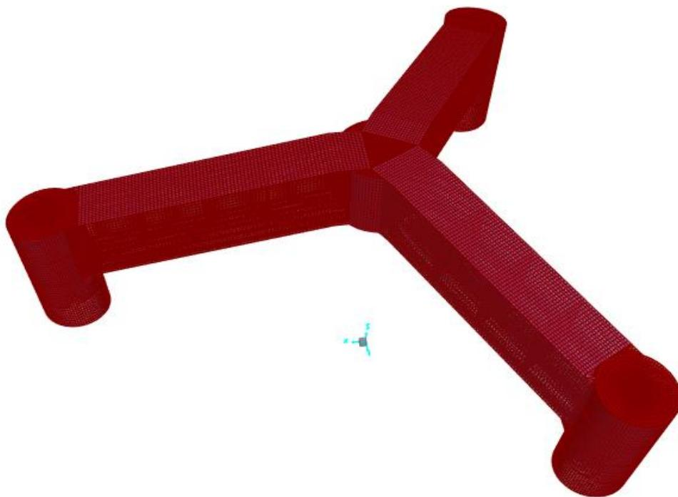
Figure 34: Overview of the FEM mesh of the steel tripod.
