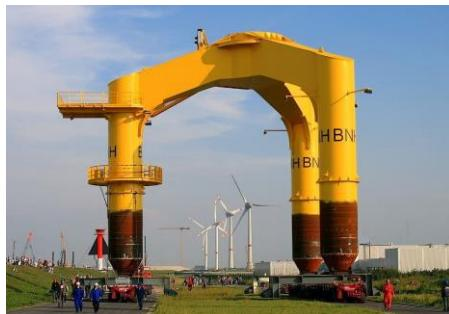
Figure 4 - Transition piece of the Bard tripile support structure.
