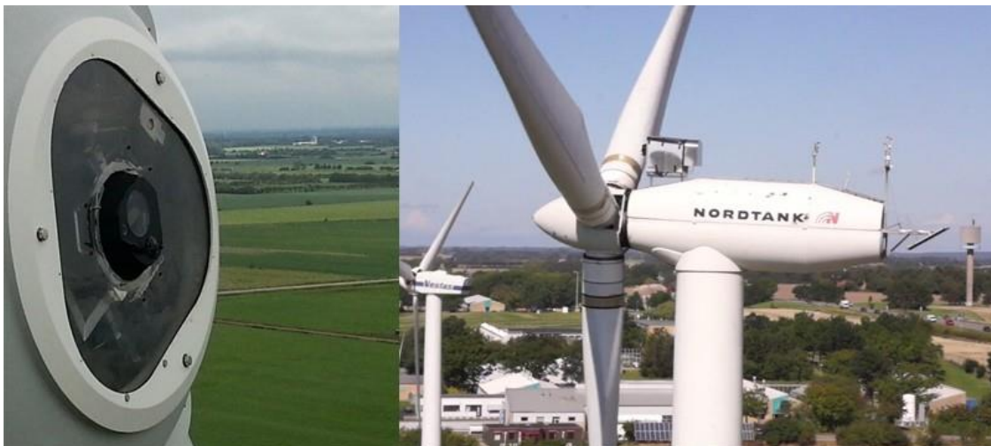
Figure 2.1: The SpinnerLidar installed (left) in a wind turbine spinner and (right) on top of a wind turbine nacelle.
