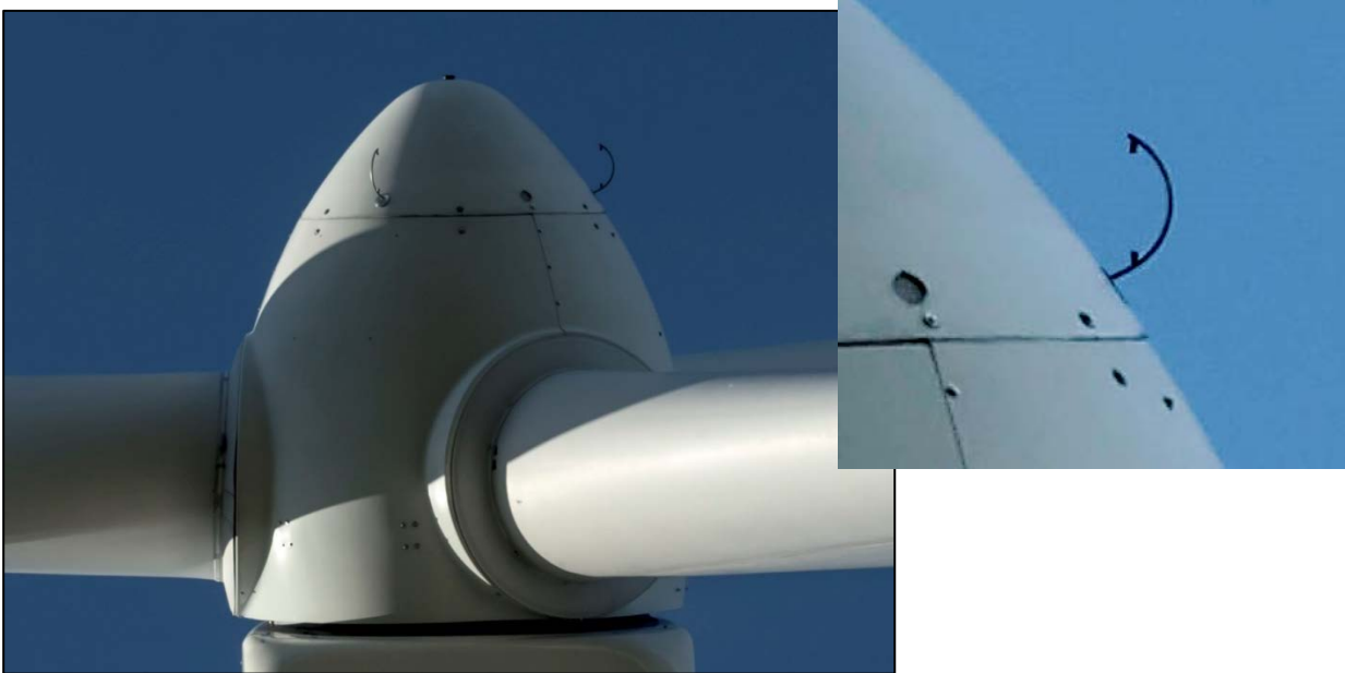
Figure 33 Installed spinner anemometer on experimental DTU wind turbine Vestas V52 showing two sonic sensors. One sensor shows the tilted sonic path in order to avoid sensor head flow distortions
