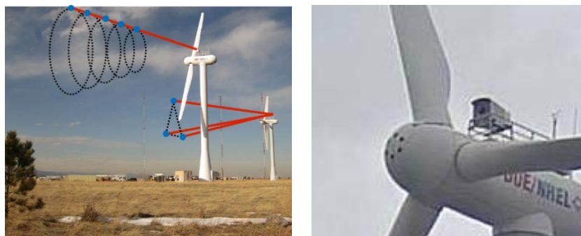
Figure 47: First field testing of lidar-assisted control at NREL (left), DTU scanning lidar system was installed from February 2014 through October 2015 on the nacelle of the CART3 (right).
