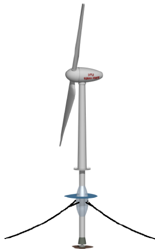
Figure 24 - Illustration of the two bladed rotor mounted on the semi-floater.
