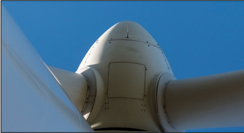
Figure 32 Installed spinner anemometer on experimental DTU wind turbine Vestas V52 showing one sonic sensor mounted in line with the shaft axis
