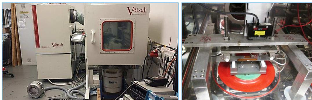
Figure 9: Four-point bending test set up
