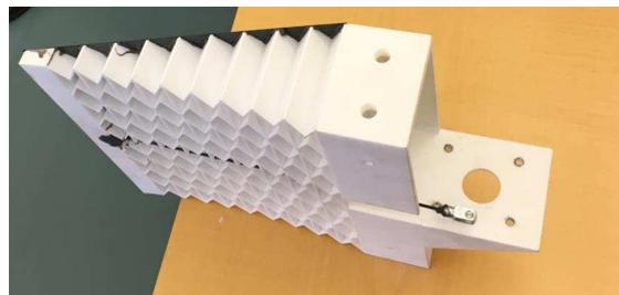
Figure 3, (Left) Rotating test-rig at DTU, Campus Risoe. (Right) A flap prototype. The silicone skin on the pressure side is not glued on at this stage. The actuation rod is visible at the lower part of the flap.
