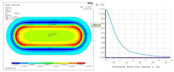
Fig. 4 FE plot of magnetic field applied to the coil
