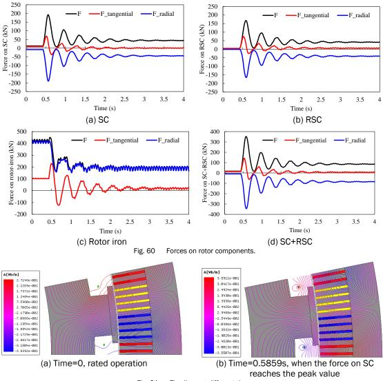
Fig. 61 Flux lines at different time.
