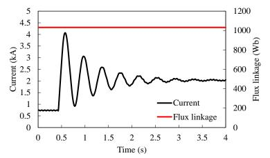
Fig. 59 Variation of field current and flux linkage with time.
