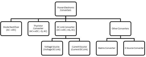
Fig. 12 Classification of power electronic converters
