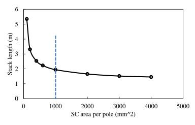
Fig. 70 Variation of stack length with SC area per pole, T=30 MNm.
