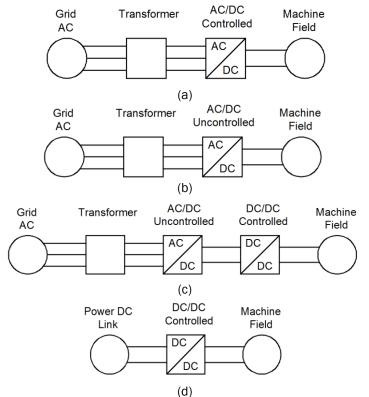
Fig. 90 Field converter topologies. (a) AC/DC controlled converter (b) AC/DC uncontrolled converter (c) AC/DC uncontrolled converter + DC/DC controlled converter and (d) DC/DC controlled converter
