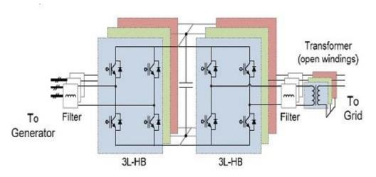
Fig. 15 Three-level H-bridge back-to-back converter for wind turbines (3L-HB BTB) [BLA10]
