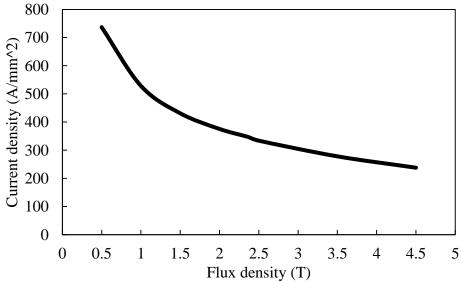
Fig. 93 Variation of engineering critical current with normal flux density in SC material, temperature=30K.
