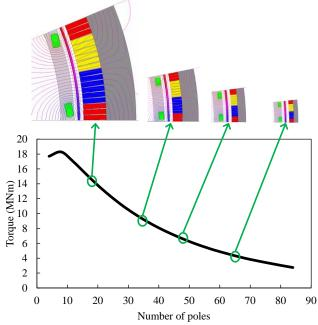
Fig. 112 Variation of torque with pole number. The optimized parameters include  $b_s$ ,  $h_s$ , and  $J_{SC}$ ; Optimization condition:  $b_{sc}/h_{sc}=2$ ,  $P_{Cu}=200$ kW,  $S_{SC}/pole=291600/(2p)$  mm<sup>2</sup>.
