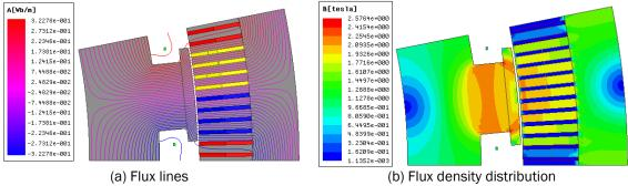
Fig. 45 Flux lines and flux density distribution under no load operation.
