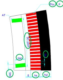
Fig. 97 Cross section and parameters of SC generator with air-core stator and rotor topology, the circled parameters are to be investigated.
