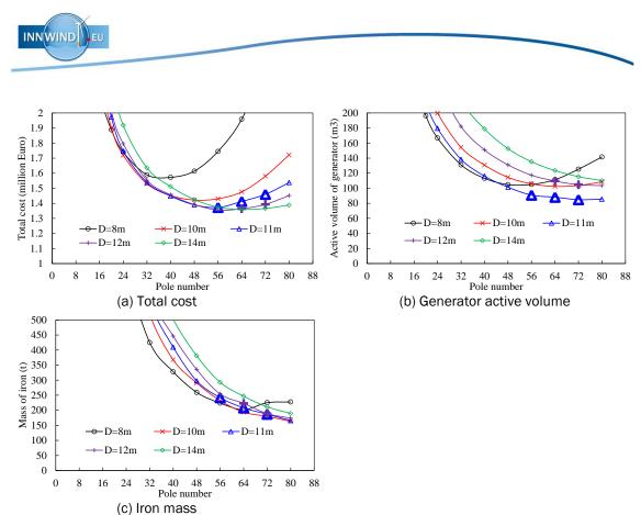
Fig. 78 Variations of active material cost, generator active volume and iron mass with pole number for different stator outer diameters, torque=30MNm.
