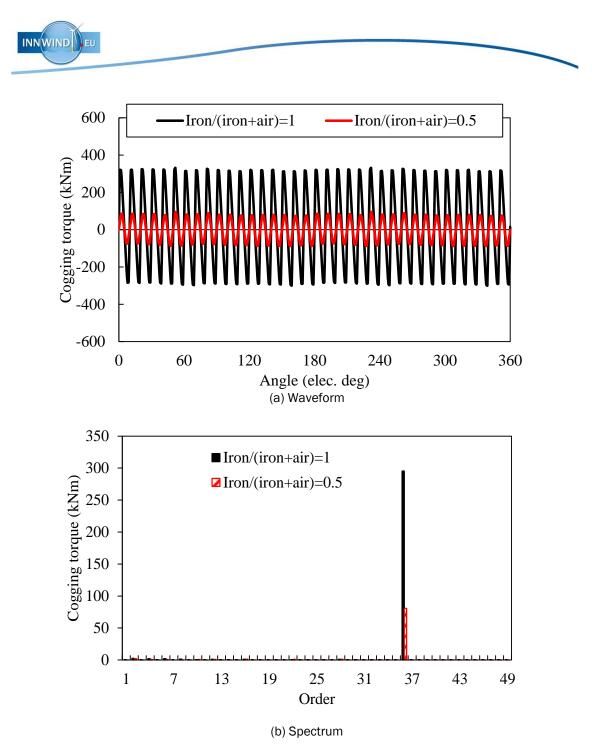
Fig. 132 Waveforms and spectrums of cogging torque.
