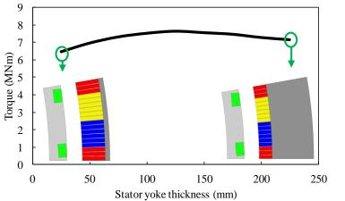
Fig. 104 Variation of torque with stator yoke thickness. The optimized parameters include  $b_{sc}$ ,  $h_{sc}$ ,  $b_{s}$ , and  $h_{s}$ ; Optimization condition:  $P_{cu}$ =85kW,  $S_{sc}$ /pole=3000mm<sup>2</sup>,  $J_{sc}$ =300A/mm<sup>2</sup>.
