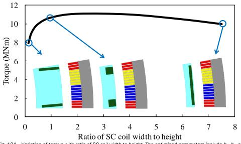
Fig. 121 Variation of torque with ratio of SC coil width to height. The optimized parameters include  $b_s$ ,  $h_s$ , and  $J_{SC}$ ; Optimization condition:  $P_{cv}$ =200kW,  $S_{SC}$ /pole=8090mm<sup>2</sup>.
