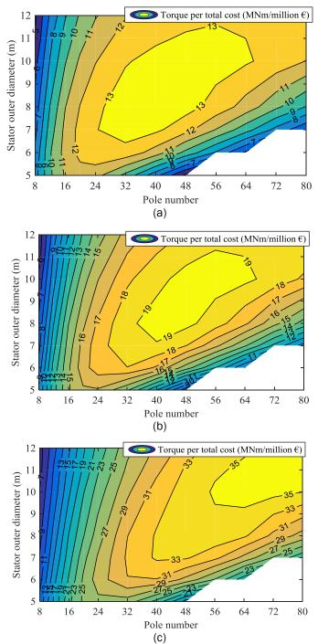
Fig. 31 Torque per active material total costs, (a) SC=100€/m, (b) SC=60€/m, (c) SC=20€/m.
