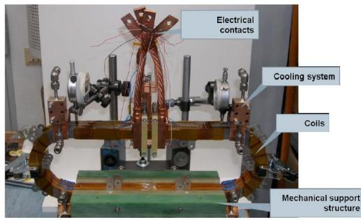
Figure 1. Final field coil before testing of critical current
