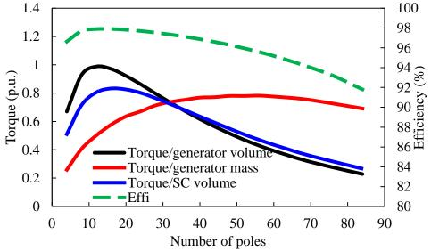
Fig. 119 Variations of torque per generator volume, torque per generator mass (only iron mass included), torque per SC volume and efficiency with pole number. The base values for torque per volume, per mass and per SC volume are 0.3MNm/m³, 0.3MNm/t, 30MNm/m³ respectively.
