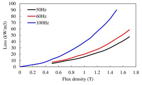
Fig. 94 Variations of losses with flux density of 50JN600
