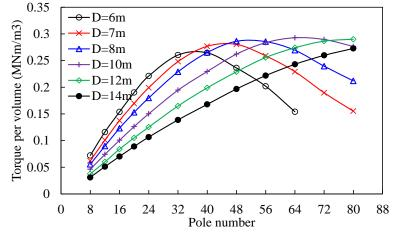
Fig. 72 Variations of torque per generator volume with pole number for different stator outer diameters, without SC end length.
