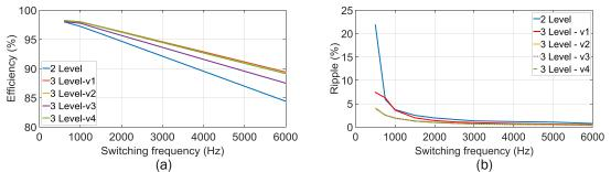
Fig. 87 (a) Efficiency and (b) torque ripple vs. switching frequency for different converter topologies (two and three level) and different switching sequences.
