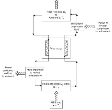
Fig. 67 A typical cryogenic system [MEL12].
