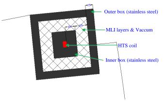
Fig. 66 Cross section of rotor pole cryostat
