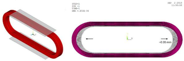
Fig. 6 Deformation in supported coil at rated current
