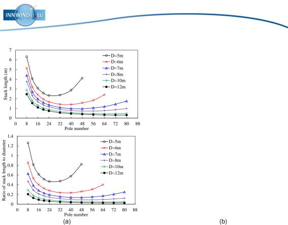
Fig. 25 Variations of stack length and ratio of stack length to stator outer diameter with pole number for different stator outer diameters, torque=10.5MNm.
