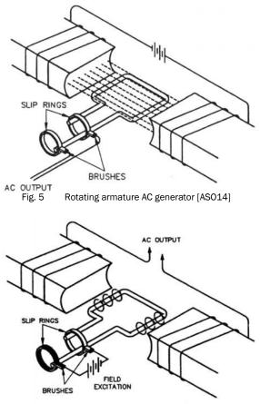
Fig. 6 Rotating field AC generator [AS014]
