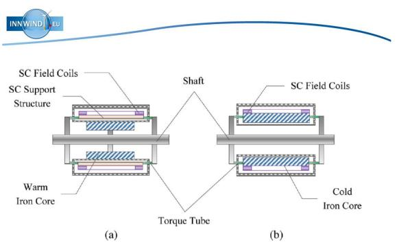
Fig. 3 Warm and cold rotor iron-core topologies. (a) Warm rotor iron-core. (b) Cold rotor iron-core. [QU13]
