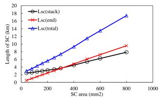
Fig. 35 Variations of SC wire length with SC area per pole, T=10.5MNm.
