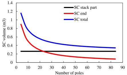
Fig. 115 Variation of SC material volume with pole number, SC stack part is the straight section of SC coil, SC end is the end section of SC coil, SC total means the whole SC coil.
