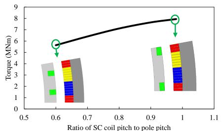
Fig. 107 Variation of torque with SC coil pitch. The optimized parameters include  $b_{sc}$ ,  $h_{sc}$ ,  $b_s$ , and  $h_{yi}$ ; Optimization condition:  $P_{Cu}$ =85kW, S<sub>SC</sub>/pole=3000mm<sup>2</sup>,  $J_{sc}$ =300A/mm<sup>2</sup>.
