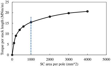
Fig. 69 Variation of torque with SC area per pole.
