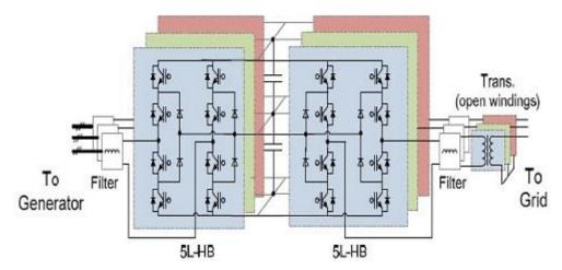
Fig. 16 Five-level H-bridge back-to-back converter for wind turbines (5L- HB BTB) [BLA10]
