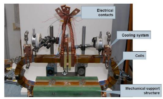
Fig. 9 Picture of the finished field coil with support structure, cooling contacts and current leads
