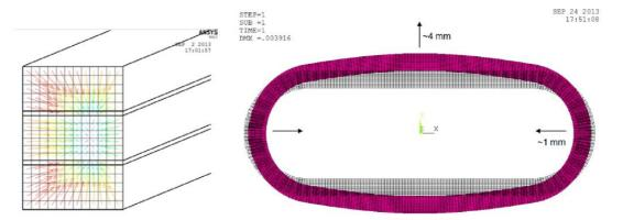
Fig. 5 forces in coil cross section and coil deformation under rated current
