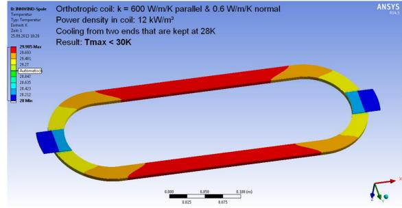
Fig. 8 Thermal distribution in the field coil under load with conduction cooling at ends of race track (blue)
