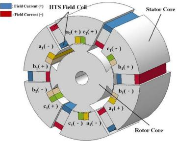
Fig. 9 Topology of flux-switching SC generator, [HWA14]
