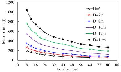
Fig. 73 Variations of iron mass with volume with pole number for different stator outer diameters, L=1m.
