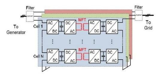
Fig. 18 Cascade H-bridge back-to-back converter for wind turbines with Medium Frequency Transformer (CHB-MFT) [BLA10]
