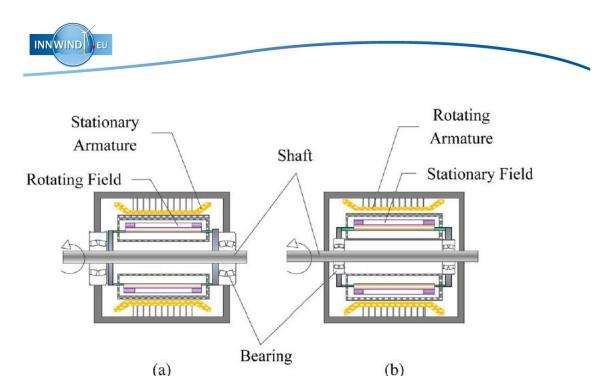
Fig. 7 Rotating armature and rotating field winding topologies. (a) Rotating armature winding. (b) Rotating field winding. [QU13]
