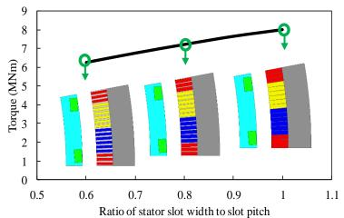
Fig. 98 Variation of torque with ratio of stator slot width to slot pitch. The optimized parameters include  $b_{sc}$ ,  $h_{sc}$ ,  $h_{s}$ , and  $h_{yi}$ ; Optimization condition:  $P_{cu}$ =85kW, Ssc/pole=3000mm<sup>2</sup>,  $J_{sc}$ =300A/mm<sup>2</sup>.
