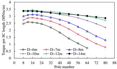
Fig. 76 Variations of torque per SC length (total length) with pole number for different stator outer diameters, T=30MNm.
