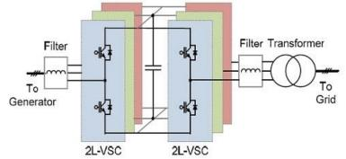
Fig. 13 Two-level back-to-back voltage source converter for wind turbines (2L BTB) [BLA10]
