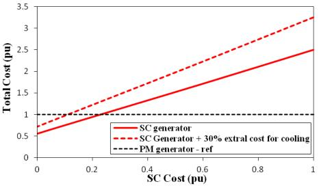
Figure 3. Comparison of active material costs for the HTS and PM DD generators
