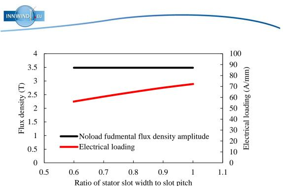
Fig. 100 Variations of amplitude of fundamental flux density in the middle of airgap and electrical loading with ratio of stator slot width to slot pitch.
