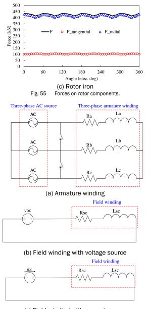
(c) Field winding with current source Fig. 56 Connections of armature and field windings.
