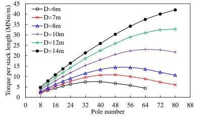
Fig. 71 Variations of torque with pole number for different stator outer diameters, L=1m.
