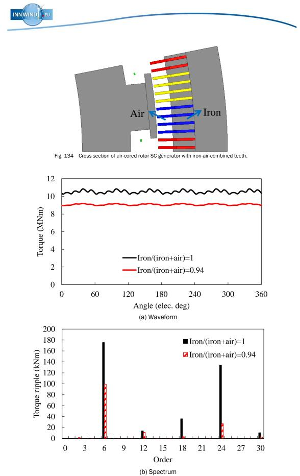
Fig. 135 Waveforms and spectrums of torque ripple, iron/(iron+air) is the ratio of iron tooth height to total tooth height.
