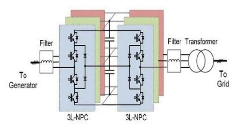
Fig. 14 Three-level Neutral Point Clamped back-to-back converter for wind turbines (3L-NPC BTB) [BLA10]
