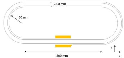
Fig. 1 Geometry layout of HTS coil with position of electrical contacts
