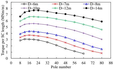
Fig. 75 Variations of torque per SC length with pole number for different stator outer diameters, without SC end length.
