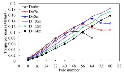
Fig. 74 Variations of T/M\_iron with volume with pole number for different stator outer diameters, without SC end length.
