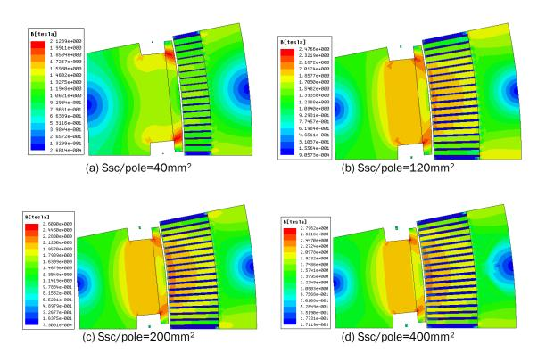
Fig. 32 Cross sections of optimized generators
