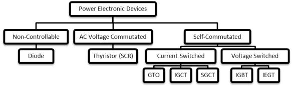
Fig. 11 Classification of the semiconductors for power electronic devices
