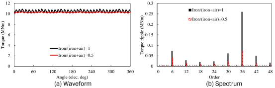
Fig. 131 Waveforms and spectrums of torque ripple, iron/(iron+air) is the ratio of iron tooth height to total tooth height.
