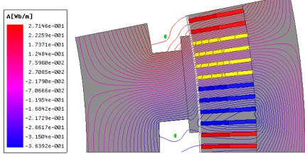
Figure 2. Cross section of the HTS generator (flux plot under load)
