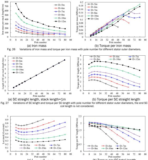
(a) L<sub>sc(stack)</sub>/L<sub>sc(total</sub>) (b) Torque per SC total length Fig. 28 Variations of ratios of SC coil straight length to total length and torque per SC length with pole number for different stator outer diameters, torque=10.5MNm.
