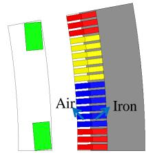
Fig. 130 Cross section of air-cored rotor SC generator with iron-air-combined teeth.
