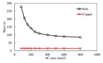
Fig. 36 Variations of iron and copper masses with SC area per pole, T=10.5MNm.
