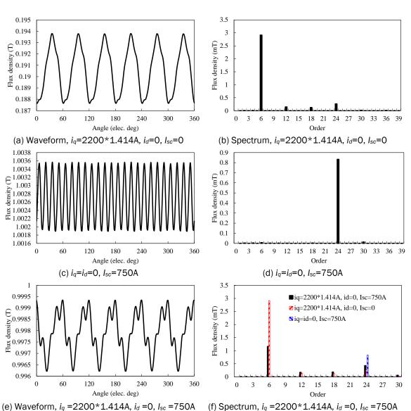
Fig. 52 Flux density waveforms and spectrums for point A in SC coil.
