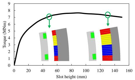
Fig. 101 Variation of torque with stator slot height. The optimized parameters include  $b_{sc}$ ,  $h_{sc}$ ,  $h_{sc}$ ,  $b_{s}$ , and  $h_{yi}$ ; Optimization condition:  $P_{cu}$ =85kW,  $S_{sc}$ /pole=3000mm<sup>2</sup>,  $J_{sc}$ =300A/mm<sup>2</sup>.
