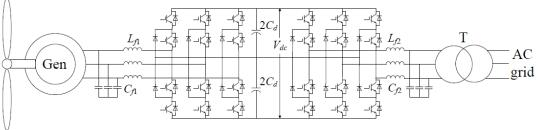
Fig. 83 3-level back to back neutral point clamped voltage source converter [INN14]
