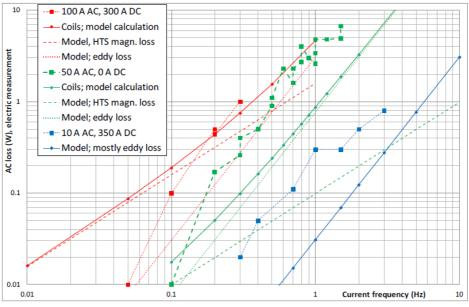
Fig. 12 Measured and calculated AC loss in field coils
