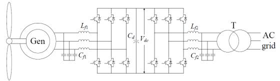
Fig. 82 2-level back to back voltage source converter [INN14]
