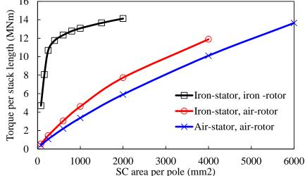
Fig. 20 Variations of torque with SC area per pole, D=7m,  $P_{cu}/stack$  length=274kW, Ja=3.5A/mm2, for each S<sub>SC</sub>/pole, the stator slot height and width, and stator yoke thickness are optimized.
