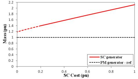
Figure 4. Comparison of mass versus HTS tape cost for cost optimised generator design
