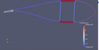
Internal structure of the optimized 10 MW design with the flap geometry - 85% blade span section. (Carlo Tibaldi)
