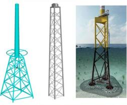
Three legged frame structures, also as a full length structure to the nacelle or for legged structures with vibration absorption devices
