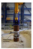
Tensile static test of Pile 2
