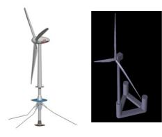
Guyed Tower with buoyancy and ballast chambers and Semi Submersible designed for a 10 MW wind turbine.
