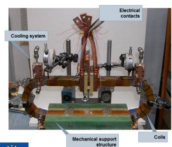
High temperature superconductor tapes
