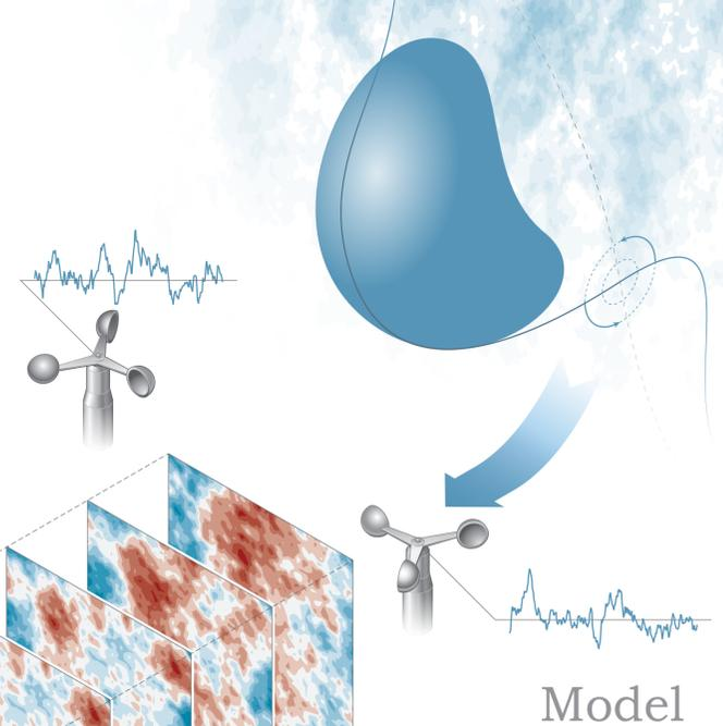
Using a sensor array makes it possible to cross-correlate wind speed measurements, which can be Fourier-transformed and matched with a **3D spectral model**. Shuffling the wave numbers and amplitudes then allows one to generate a fully stochastic turbulent velocity field. Though, when imposing certain constraints on the randomization, the field can be tailored in such a way that it contains discrete events (gusts) that satisfy certain requirements.
