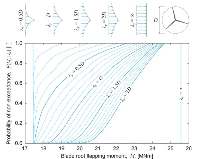
(above) Response of the DTU 10 MW reference turbine to a gust of various sizes. The size of the gust has a large impact on the variation in load output. Smaller gusts have a high probability of triggering no response at all, either by missing the rotor blades or landing close to the blade root. Striking is how even the largest gusts—here  $2D$  is equal to 357 m—remain far below the level of the uniform case.
