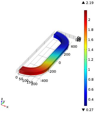
Figure 2-12 Displacement of the coil after cooling it down from room temperature to T = 30 K. The displacement is shown in the unit of [mm]. Only the coil domain is shown in the figure.
