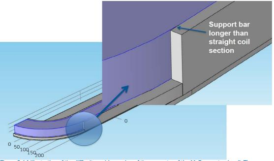
Figure 2-14 Illustration of the difficult meshing region of the geometry of the MgB<sub>2</sub> race track coil. The stainless steel support bar is extending further than the coil, but the intersection line will change as the coil is deformed resulting in a difficult meshing situation. Thus the result along the intersection line is neglected as being a mesh artifact.
