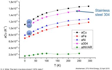
G. K. White, "Exp tech in low temp physics" (1979), table F Abrahamsen, DTU Wind Energy. 23 April 2015 Figure 2-9 Linear coefficient of expansion of different metals as function of temperature. Appropriate numbers for Cu, stain less steel and Ni at T = 30 K were used in the simulation.
