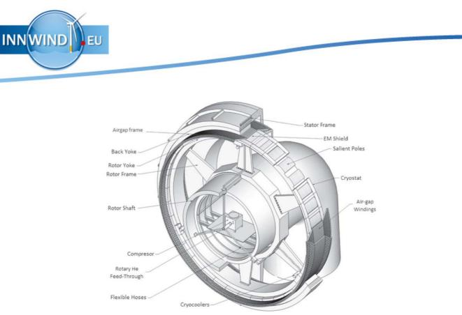
Figure 3-2 Illustration of how the helium compressor is placed in the static frame in the center of the hub and is connected to the cold heads on the inner rim of the generator. Reproduced from Fig 1 in (Marino, Pujana, & Sarmiento, 2016)
