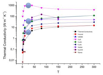
G. K. White, "Exp tech in low temp physics" (2002), table B.6 Abrahamsen, DTU Wind Energy, 23 April 2015 Figure 2-10 Thermal conductivity of construction materials used for cryogenic supports as function of temperature. Appropriate numbers for Cu, stainless steel and Ni at T = 30 K were used for the thermal stress simulation.
