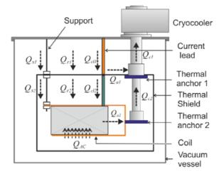
Figure 3-3 Illustration of the heat inflow of the SUPRApower cryostat. Reproduced from Fig. 5 in (Sun, Sanz, & Neumann, 2015).
