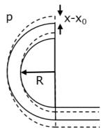
Figure 2-4 <u>Illustration of deformation of end sections of the race track coil as the straight sections are moved</u> outwards to x from x<sub>0</sub>. The perimeter of the elliptical end-section is denoted p and the minor axis of the ellipse is given by the radius R of the initial circular end section.
