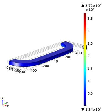
Figure 2-13 Von Misses stress in the coil due to thermal stress after cooling down the coil from room temperature to T = 30 K and conducting 1 W of heat away from the coil. The unit of the stress in [Pa] and it should be noted that the maximum of the color bar is equivalent to 372 MPa. This is however an artifact of a challenging meshing of the coil geometry, which is explained in a following graph. The Von Misses stress level is around 30 – 60 MPa. Only the coil domain is shown in the figure.
