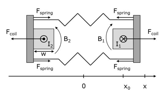
Figure 2-3 Illustration of force  $F_{coll}$  action on the two straight sections of an infinitely long race track coil, where the two conductors are holding the current  $I_2$  and  $I_2$  of equal size but opposite direction. The coil sections are supported by two plates, which are hold together by support rods providing the spring force  $F_{spring}$ .
