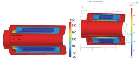
Figure 2-15 Illustration of torque tubes transmitting the generator torque from room temperature and to the support structure of the coil at low temperature of T = 20 K. Reproduced from deliverable D3.42 fig 4-5 and 4-6 (Liu, et al., 2013).
