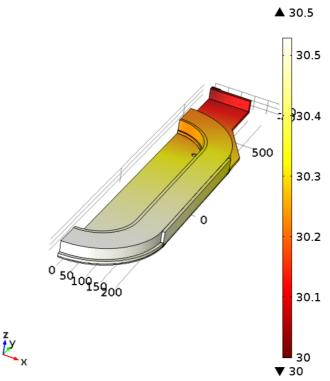
Figure 2-11 Temperature distribution of the coil and thermal support when a heat dissipation of 1 W is distributed evenly in the coil and conducted to the cold head mounted on top of the plate at the top. Only  $\frac{1}{4}$  of the geometry is calculated to improve computational efficiency. The scale is temperature [K].
