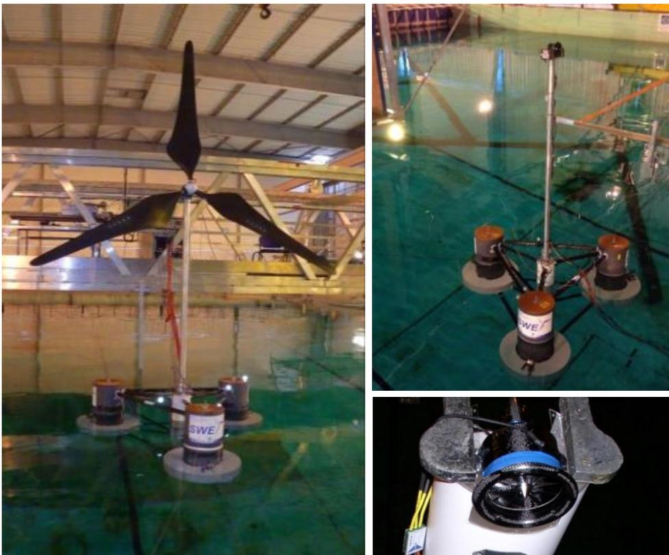
**Figure 2-8: Measurement campaign at Ecole Centrale de Nantes, France, (LHEEA). The design of the floating model is based on the OC4/DeepCWind**
