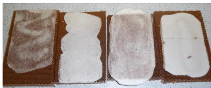
**Figure 81. Photographs of different morphing skin samples. One can notice the increasing quality of the surface of the foam. From left to right: 2:1 polyol to isocyanate mixing ratio / no release agent; 2:1.5 polyol to isocyanate mixing ratio / no release agent; 2:1.125 polyol to isocyanate mixing ratio / silicon release agent; 2:1.125 polyol to isocyanate mixing ratio / wax release agent.**
