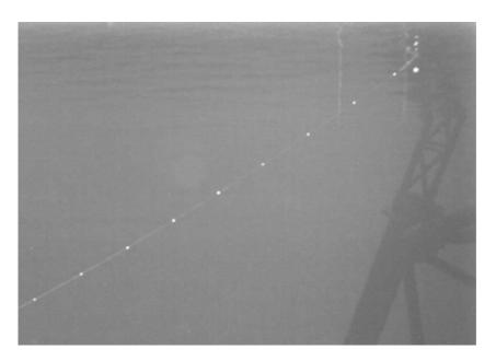
Figure 4.4: Chain with markers to measure the motions
