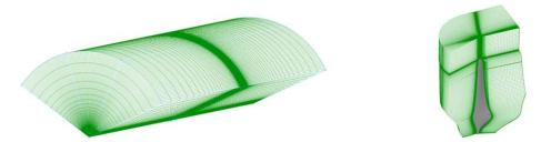
Figure 67 - Background (left) and blade (right) grid of the one third model in FLOWer
