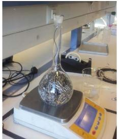
Figure 4.5: Measurement of the displaced volume of the chain
