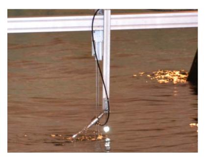
Figure 4.3: Load cell for the measurement of the tension
