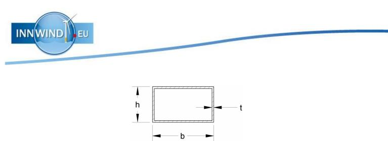
Figure 3.1-4 cross section of the main spar of the blade (Larsen, et al., 2007)
