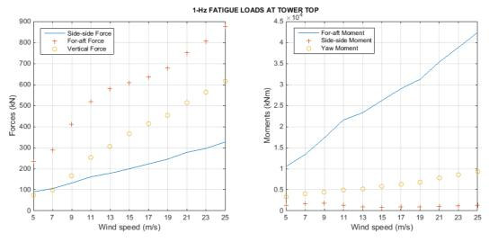
Figure 3.8-1 – 1 Hz damage equivalent load at tower top
