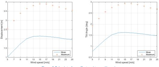
Figure 3.7-1 – Interface offset and tower tilt angle
