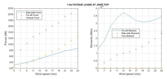
Figure 3.8-3 – 1 Hz damage equivalent load at joint top
