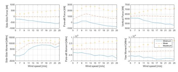
Figure 3.7-2 - Ultimate loads at tower top
