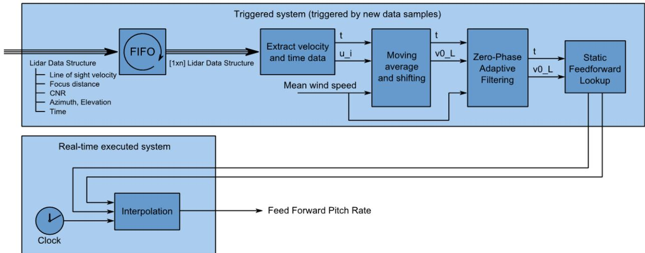
Figure 1: Schematic view of the lidar data processing for providing an estimate of the rotor effective wind speed  $v_{0L}$  to the feedforward controller.
